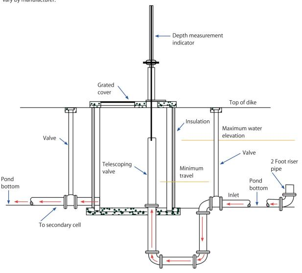
Figure 7B: **Telescoping valve**
