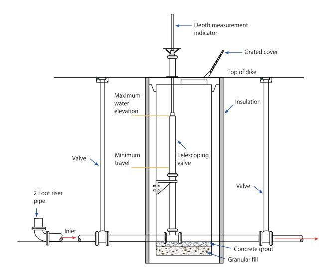
Figure 7C: **Telescoping valve**
