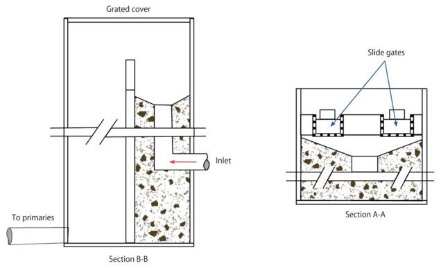
Figure 7A: **Telescoping valve**
