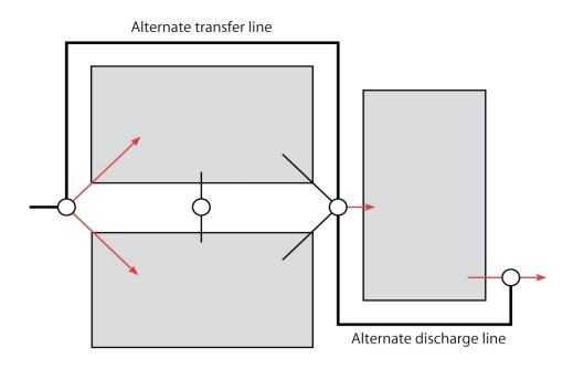
Figure 2: Two-cell non-aerated stabilization pond
