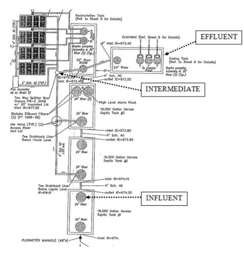
Figure 19. Flow Schematic: Whispering Ridge East WWTP
