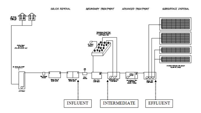
Figure 3. Flow Schematic: Diamond Lake Woods WWTP,
