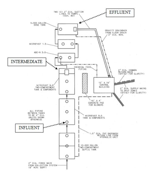
Figure 5. Flow Schematic: Farms of Lake Elmo WWTP
