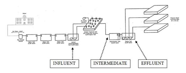
Figure 1. Flow Schematic: Cambridge-Isanti Middle School WWTP
