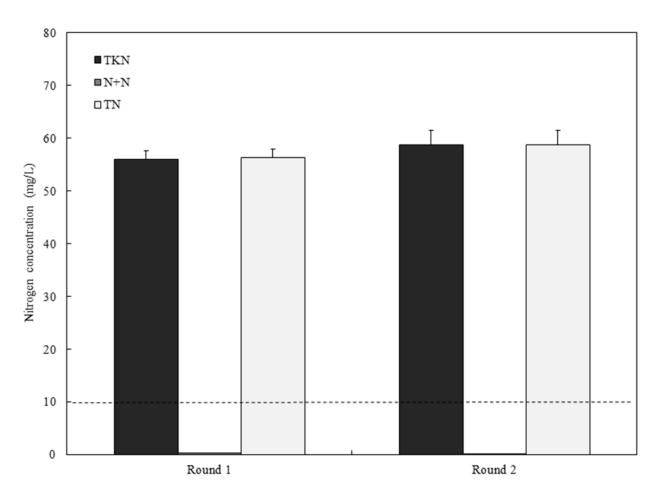
Figure 8. Effluent Nitrogen series: Preserve at Birch Lake WWTP.
