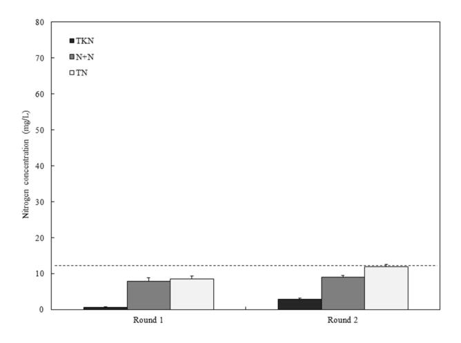
Figure 20. Effluent Nitrogen series: Whispering Ridge East WWTP.
