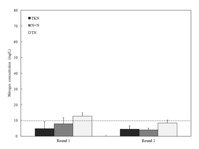
Figure 18. Effluent Nitrogen series: West Lake George WWTP.
