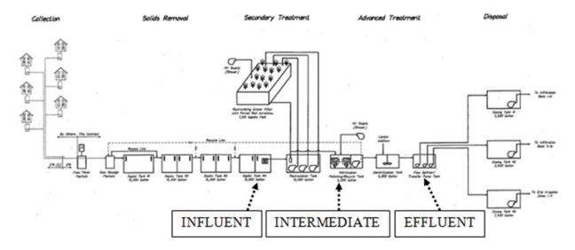
Figure 13. Flow Schematic: Sanctuary WWTP
