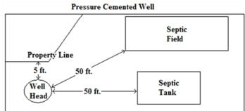
Setbacks are important – provide a margin of safety to prevent exposure to sewage contaminants
