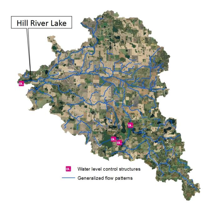
Figure 4-3: Aerial photograph (FSA 2015) of Hill River Lake (DOW 60-0142-00) and the contributing watershed. Note the location of the water level control structure on the southwestern shore; also showing three upstream water level control structures.
