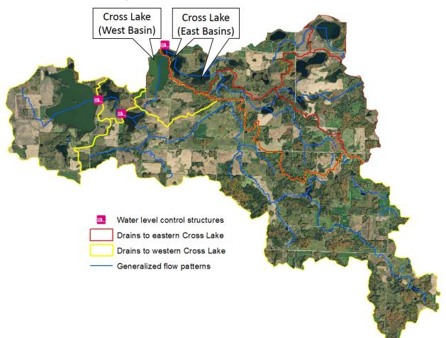
Figure 4-1: Aerial photograph (FSA 2015) of Cross Lake (DOW 60-0027-00) and the contributing watershed. Note the location of the water level control structure on the northern shore of the northern basin. The watersheds highlighted in yellow flow into the portion of Cross Lake that is sampled by MNDNR – Fisheries Personnel.
