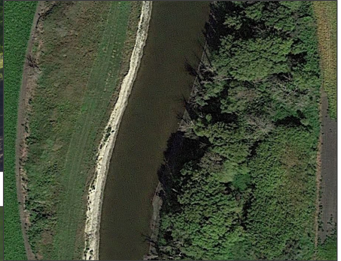
Photo 2. High, steep eroding bank on left side of channel along AUID-501.
