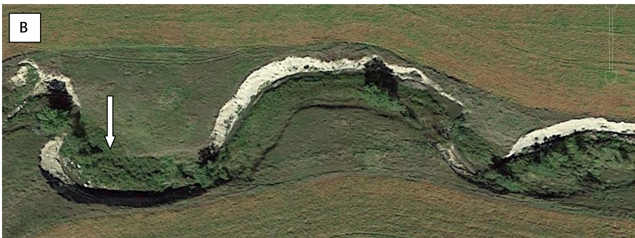
Photo 21. This location is about 1/2 to 3/4 miles upstream of Township Road 18. A) The whitish areas along the channel are raw soil banks that are eroding, which is occurring on both the ditched section on the right and the non-ditched section on the left side. B) A closer view of part of photo A, showing the steepness and height of the raw banks. Note the small size of the baseflow channel (arrow) relative to the actively-eroding valley.
