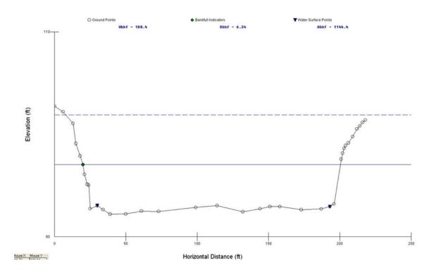
Figure 143: Riffle cross section on the Cedar River.
