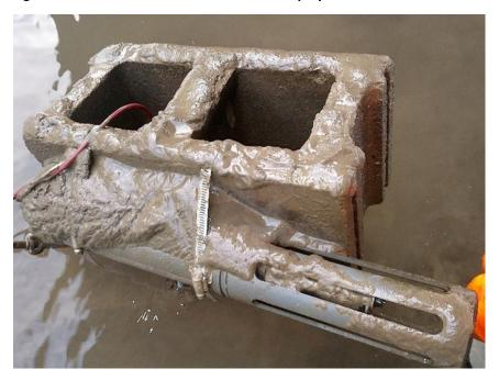
Figure 15. Sediment accumulation on sonde deployed at 15LM043 for two weeks at the end of August 2017.
