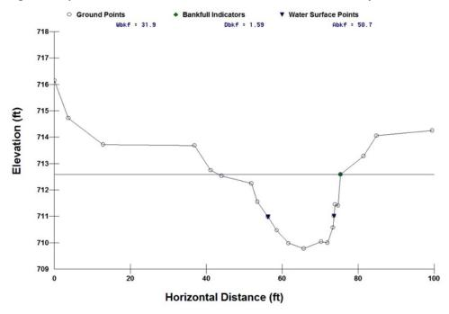
Figure 5. Representative riffle cross-section from the downstream survey location.
