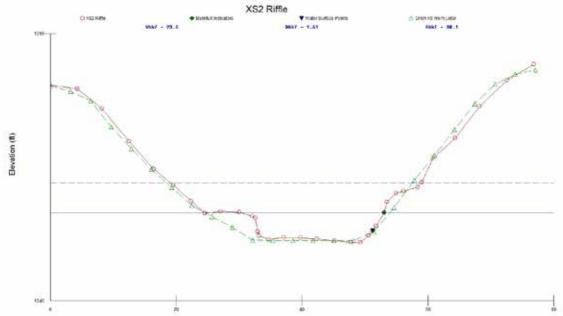
Figure 95. Riffle cross section (red) with LiDAR (2011) overlay (green).
