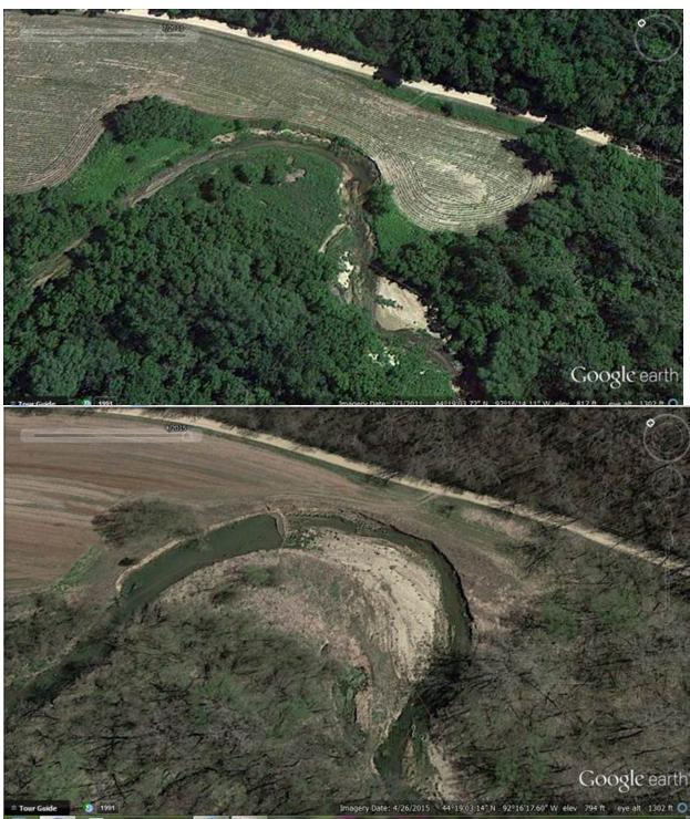
Figure 33. Meander migration over an approximate four-year time period in Spring Creek (Imagery 2011 compared to 2015) showing excessive bank erosion in areas with little vegetative protection.
