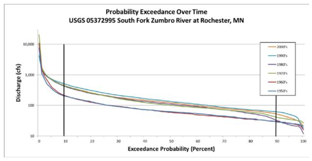
Figure 17. Flow Duration curve developed from data on the South Fork Zumbro River at Rochester, Minnesota for the period of record. Duration curves were computed for each decade on record to show the changes over time over the entire range of flows for the site.
