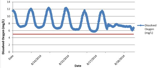
Figure 143. Continuous DO monitoring at the 45<sup>th</sup> St Crossing along Cascade Creek (0704004-991)
