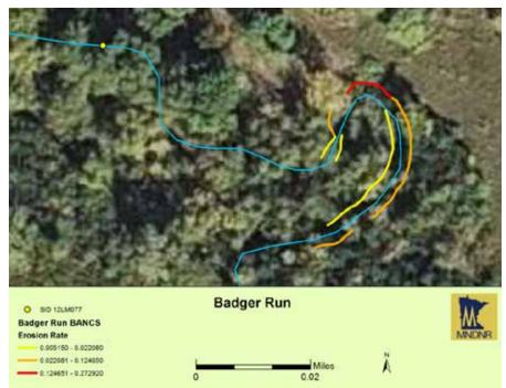
Figure 130. Erosion rates of Badger Run near site 12LM077.
