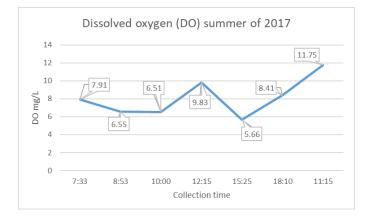
In 2018 DO monitoring took place at the outlet of Elm Creek (17MN327). Samples were of concern as all measurements collected fell close to the 5 mg/L threshold.
