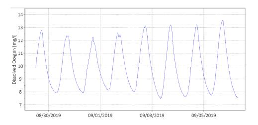
Dissolved oxygen was recorded closely together over the months of Late August and Septemer. The Fist continuous DO reading did not result in any reading below the 5 mg/L threshold for aquatic life. However, there was some extreeme 24 hour DO flucuation. Typically the 24 hour DO change ranged from 4 mg/L – 7 mg/L.
