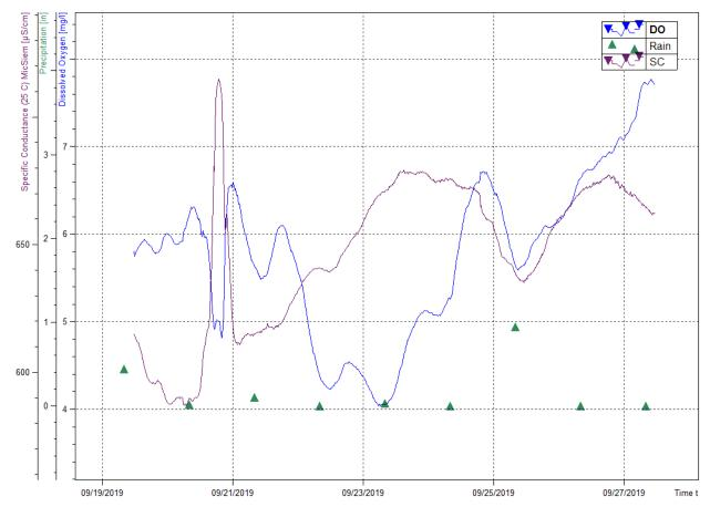
Figure 25. Continuous DO recorded with precipitation, and specific conductance at 17MN301.
