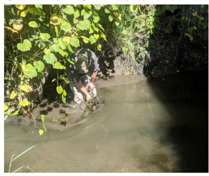
Figure 28. Sonde with fowling at the time of pick up at 17MN354.
