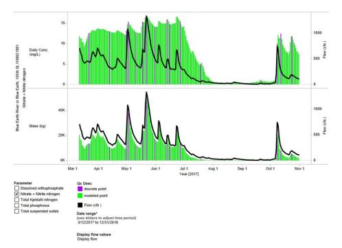
Figure 72. Nitrate concentrations with flow in the Blue Earth River at WPLMN site near the town of Blue Earth. Purple shows measured concentrations while green is modeled, black line indicates flow.
