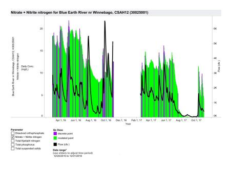
Figure 124. WPLMN station near Blue Earth, showing measured nitrate in relation to flow within the Blue Earth Subwatershed.
