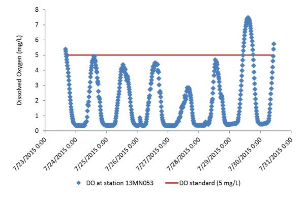
Figure 102. Continuous dissolved oxygen measurements (mg/L) at 13MN053 from July 23, 2015 to July 31, 2013.
