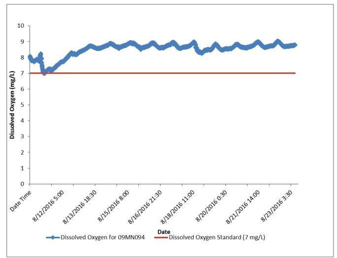
Figure 98. Continuous dissolved oxygen measurements (mg/L) at 09MN094 from August 12, 2016 to August 23, 2016.
