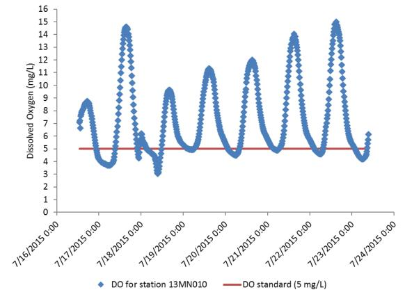
Figure 206. Dissolved oxygen flux for station 13MN010, July 17 – 22, 2015.
