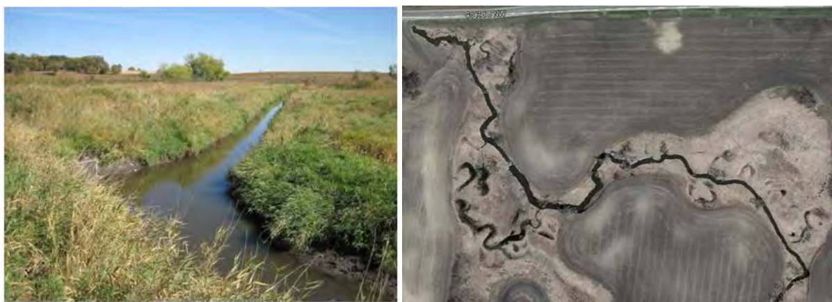
Figure 638-9: Upstream ditching and meander cutoffs
