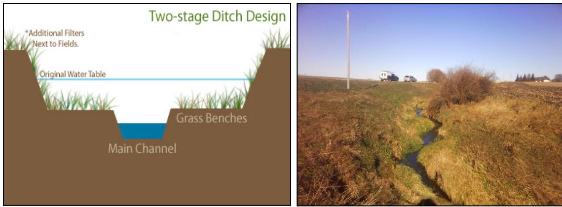
Figure 91: Cross-section of design for two-stage ditch (left) and natural forming two-stage ditch (tributary to Grove Creek in NF Crow watershed)
