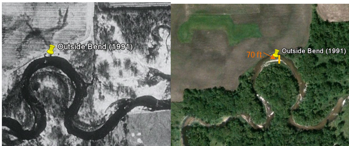
Figure 94: Aerial photos of an outside bend of the NF Crow River near Forest City, MN. A cultivated field is adjacent to the river without any vegetated riparian buffer. Comparing aerial photos from 1991 to 2009 reveals about 70 feet of lateral migration in the stream channel, for an average of about 3.9 ft of eroded bank per year
