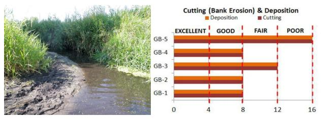
Figure 13: Example of accelerated point bar development from excess sediment deposition at station GB-5. Graph shows PSI metric scores (4 = Excellent, 16 = poor)
