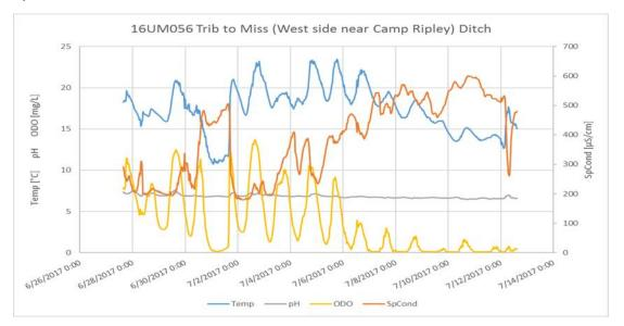
Figure 13: YSI sonde deployment at 16UM056 from June 27-July 12, 2017. Note that "ODO" in the graph represents DO.
