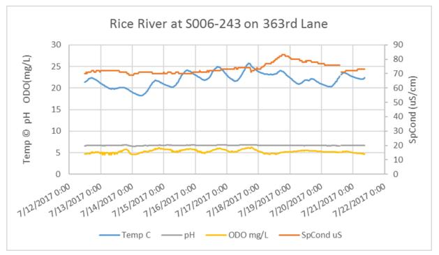
Figure 45: Sonde deployment for 9 days in July of 2017 at 363<sup>rd</sup> St. crossing on the Rice River.
