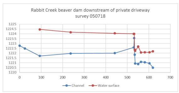
Figure 41: Longitudinal stream elevation survey from the private driveway north of Hwy 47. Survey goes downstream for 625 feet past a major beaver dam on channel.
