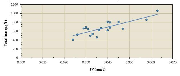
Figure 55. Correlation of TP with Total Iron in TSHL at S009-506. The regression line has R<sup>2</sup> of 0.6554.
