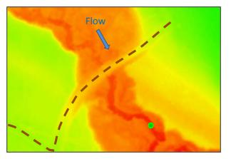
Figure 33. BANCS categorizations of streambank sections a short distance downstream of 16UM167. Colors represent categories of estimated sediment input from a given stream bank section. Bank erosion estimates increase as colors move from green to yellow to orange to red to pink.
