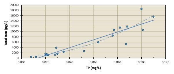
Figure 47. Correlation of TP with Total Iron in Musselshell Cr. at S009-505. The linear regression line has R<sup>2</sup> of 0.8434, while the power regression line (dotted) has R<sup>2</sup> of 0.8669.
