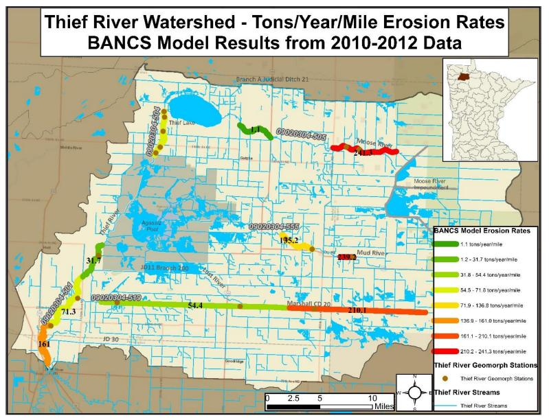
Figure 2-16. BANCS Model stream bank erosion predictions from the Thief River Watershed Fluvial Geomorphology Report. The circles and ovals encompass the reaches that were evaluated.
