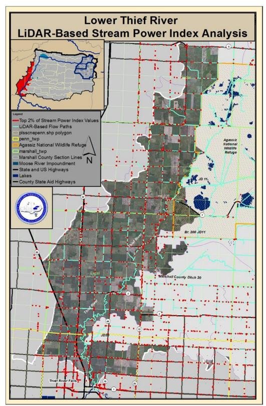
Figure 3-5. Lower Thief River Watershed high erosion potential based upon the top 2% of stream power index values.
