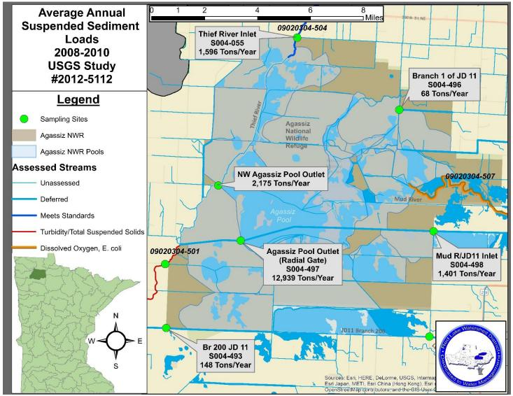
Figure 2-18. Average annual sediment loads (2008-2010 Tons/Year) from the USGS Assessment of Nutrients and Suspended Sediment Conditions in and near the Agassiz National Wildlife Refuge, Northwest Minnesota, 2008-2010 study.
