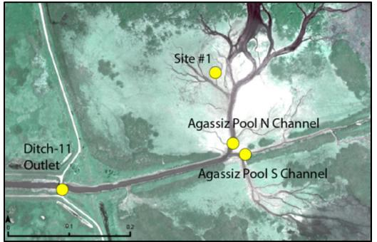
Figure 2-28. Scouring of sediment and gully formation within Agassiz Pool (Eash 2012)
