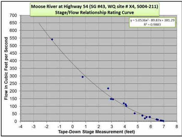
Figure 2-35. Moose River at Highway 54 (S004-211) Flow Rating Curve
