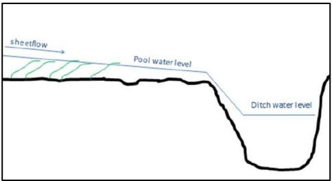
Figure 2-30. Diagram of hypothetical water surface profile within Agassiz Pool during periods of sheet flow (Eash 2012).
