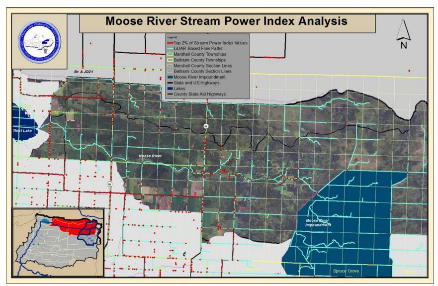
Figure 3-6. Moose River Watershed high erosion potential based upon the top 2% of stream power index values.
