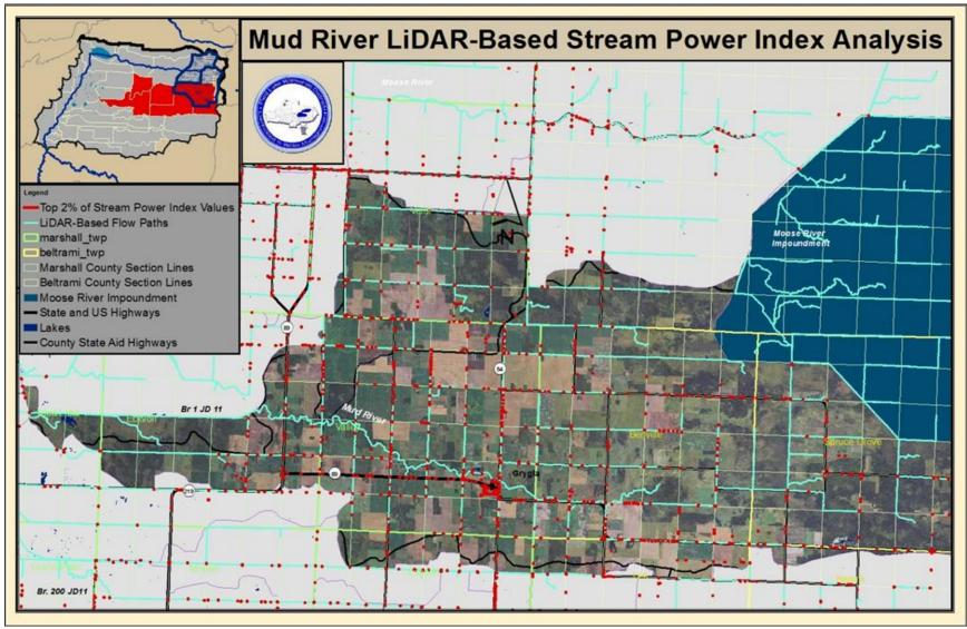
Figure 3-7. Mud River Watershed high erosion potential based upon the top 2% of stream power index values.
