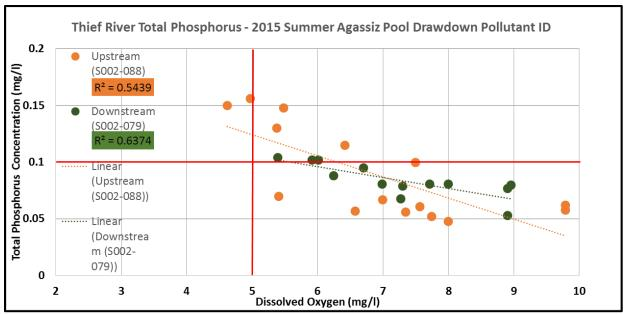
Figure 2-33. The strength of the correlation (R<sup>2</sup>) between dissolved oxygen and total phosphorus increases from the upstream end of the reach to the downstream end of the 09020304-501 reach of the Thief River.
