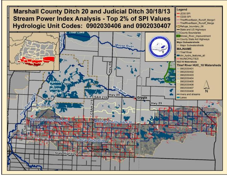
Figure 3-10. Marshall County Ditch 20 and JD30/18/13 Watersheds - high erosion potential based upon the top 2% of SPI values.
