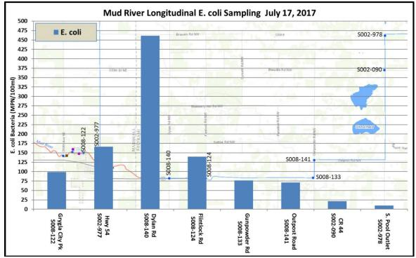
Figure 3-13. July 17, 2017 longitudinal E. coli sampling results along the Mud River upstream of Grygla.
