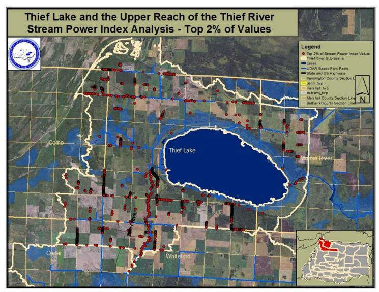
Figure 3-8. Thief Lake and upper Thief River Watershed high erosion potential based upon the top 2% of stream power index values.
