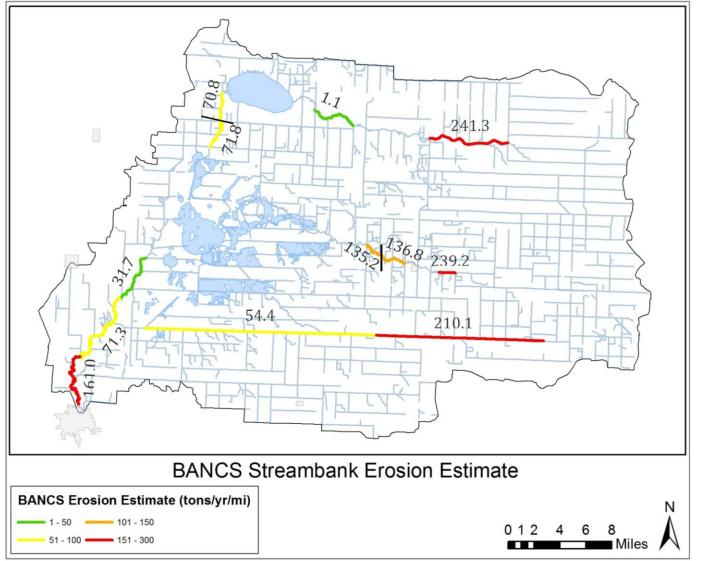
Figure 3-16. Stream bank erosion predictions from the BANCS model
