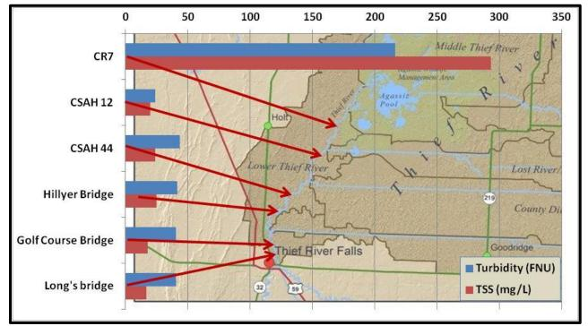
Figure 2-22. Longitudinal turbidity and TSS levels during a May 20, 2013 runoff event
