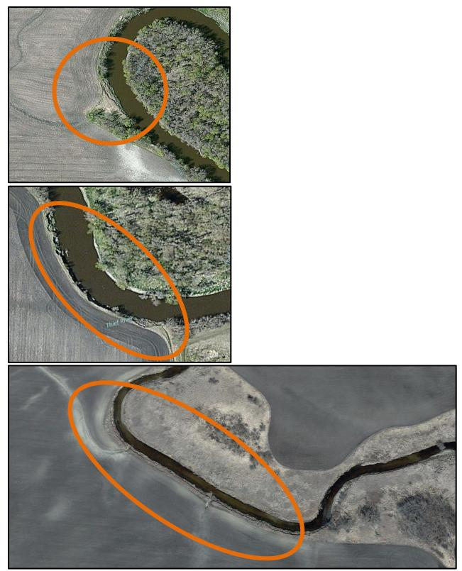
Figure 2-15. Examples of streambanks along the lower Thief River (top two photos) and the Mud River (bottom photo) that were badly eroding due to a lack of a buffer and a lack of deep-rooted vegetation
