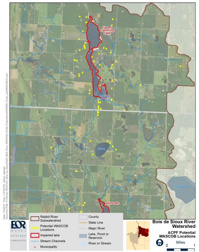
Figure 24. Potential sedimentation basin (WASCOB) locations in the Ash and Upper Lightening Lakes drainage areas
