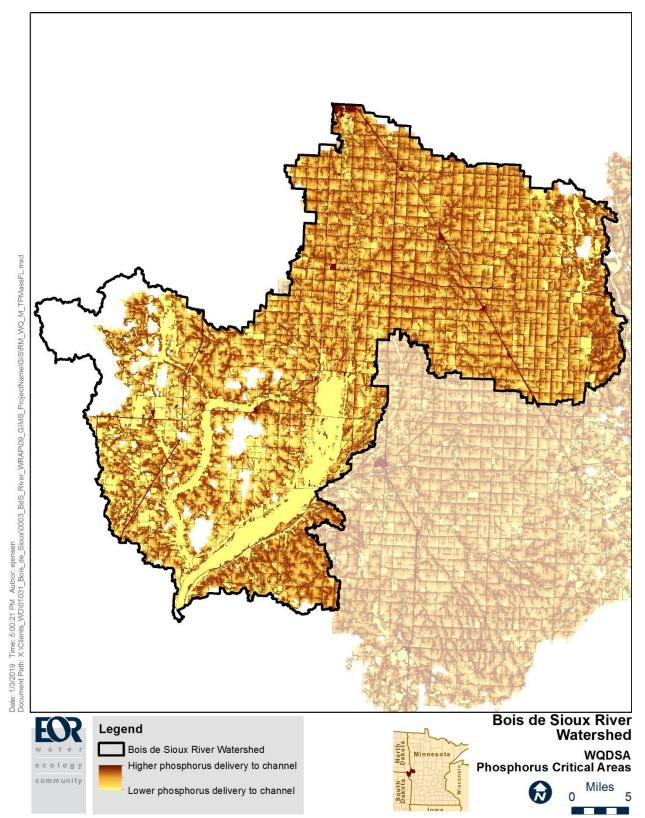
Figure 11. WQDSA Phosphorus Critical Areas in the Bois de Sioux River Watershed (darker shading denotes higher phosphorus delivery to the stream channel)
