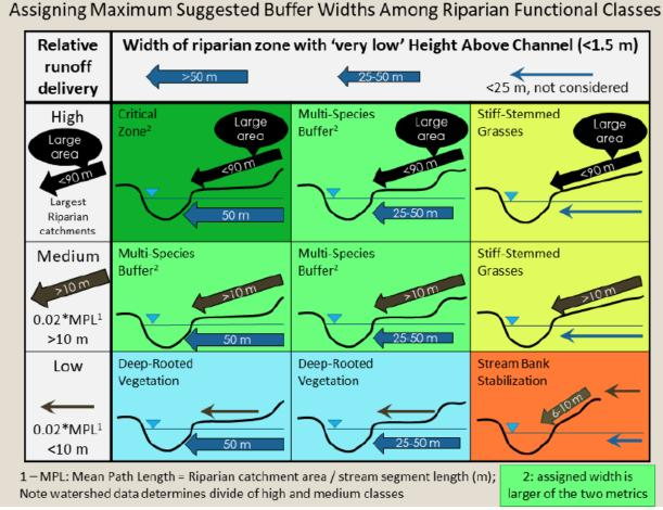
Figure 14. Graphical depiction of assigning maximum suggested buffer widths and vegetation type, based on the riparian segment classification (Figure 14 from the Agricultural Conservation Planning Framework ArcGIS Toolbox User's Manual Version 3.0. Date of Release: 08/2018).
