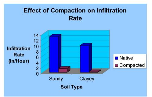
Figure 57. Infiltration rates by soil type and level of compaction. (Source: Minnesota Stormwater Manual)
