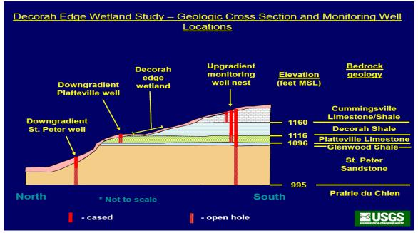
Figure 27. Decorah Edge study wells. The data in this figure are from the shallow wells with the open hole interval in the Cummingsville Limestone. Figure from Jones et al.
