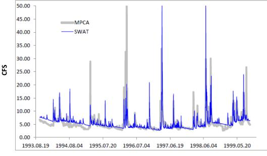
Figure 39: Whitewater Watershed Hydrologic Calibration (1993-1999). "MPCA" data includes all observed data and was provided to EOR by the MPCA.
