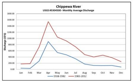
Figure 29: Comparison of Monthly Average Discharge and between two time periods at Highway 40
