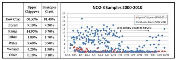
Figure 6: Comparison of NO2-3 samples (ppm) by date from two separate sub-basins of the Chippewa River Watershed
