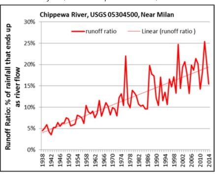
Figure 28: Runoff ratio over time. Data Sources: USGS and UMN.
