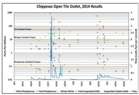
Figure 33: Delivery of water, nutrients and TSS from tile line flow
