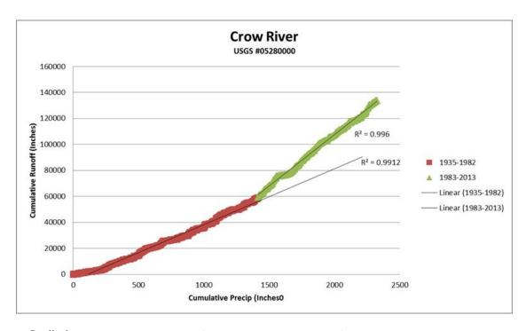
Figure 1: **Preliminary** Double Mass Curve for the Crow River at Rockford, showing the relationship between precipitation and river discharge.
