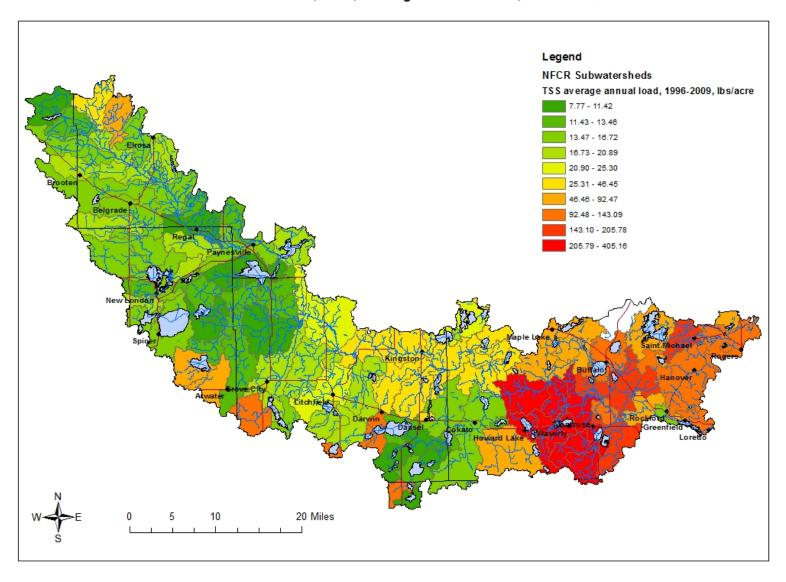
Figure 6. Sediment loading by sub-watershed in the NFC watershed
