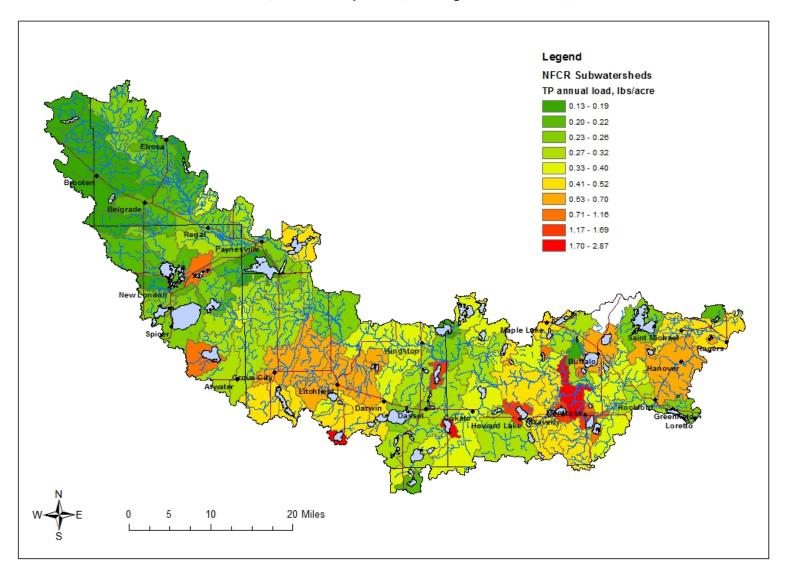
Figure 5. Total phosphorous loading by sub-watershed in the NFC watershed
