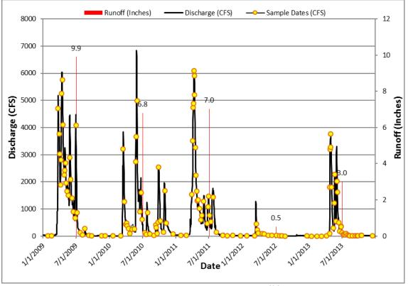
Figure 16. 2009-2013 hydrograph, sampling regime and annual runoff for the Two River near Hallock, Minnesota.
