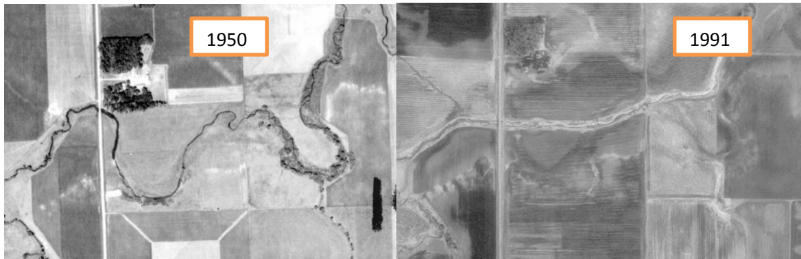
Figure 24. The channel at the North Fork Watonwan geomorphology survey site was straightened at some point between 1950 and 1991.
