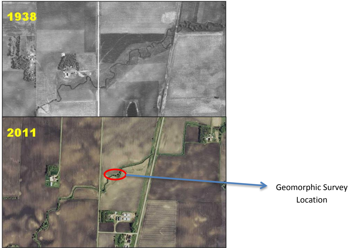
Figure 39. Aerial photography depicts historical channelization of the upper St. James Creek geomorphology survey site.
