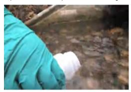
Fill the lab's collection bottle with sufficient volume as instructed by the lab.
