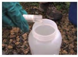
Once filled, cap the sample bottle, ensure your name and the sample collection date, location, and time are on the label, and place it inside a re-sealable plastic bag. Place the bag into a cooler and prepare the cooler for pickup or shipment to the lab. This will include packing the sample with ice (not ice packs. They cannot uniformly surround the sample bottle).
