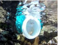
Collect the sample from as close to the middle of the stormwater flow as possible; this provides the most representative sample of that discharge.
