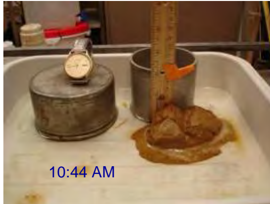
Figure 12: Time series pictures of a clod showing its disintegration when placed in shallow water.
