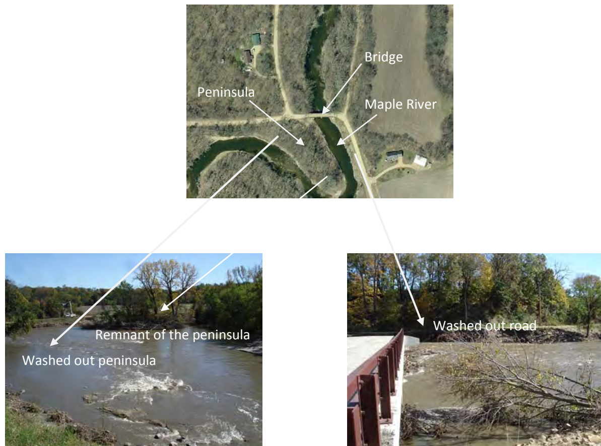
Figure 16: A peninsula in the Maple River near Good Thunder. The peninsula as well as road connecting the bridge washed out due to heavy rainfall (25 cm in a day) in the area in September 2010.
