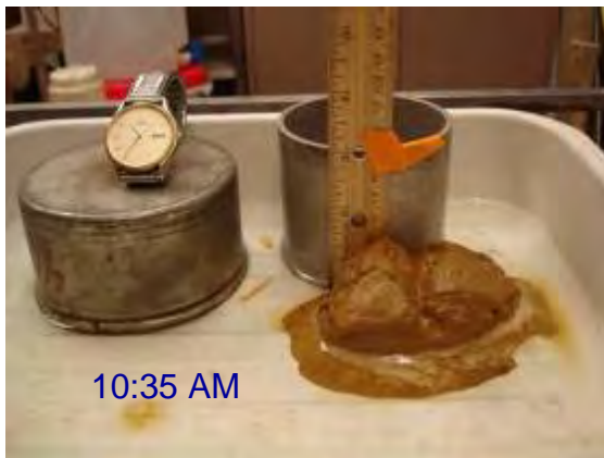
Figure 12: Time series pictures of a clod showing its disintegration when placed in shallow water.
