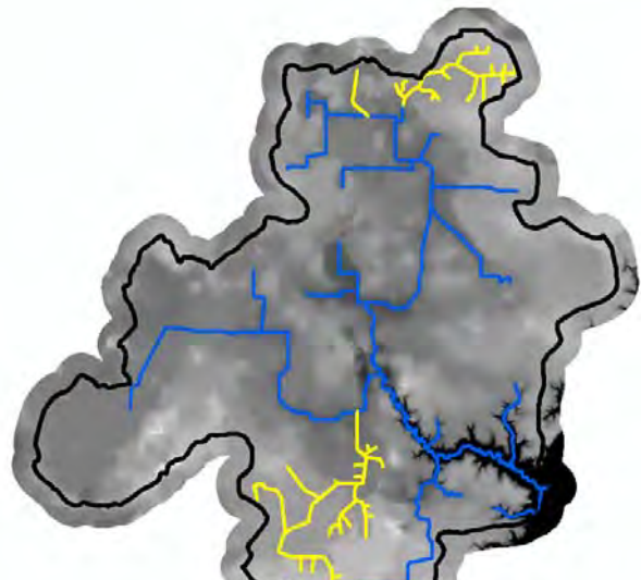
Figure B-2. Map showing the location of public subsurface drainage (yellow) which was used to aid in watershed delineation.
