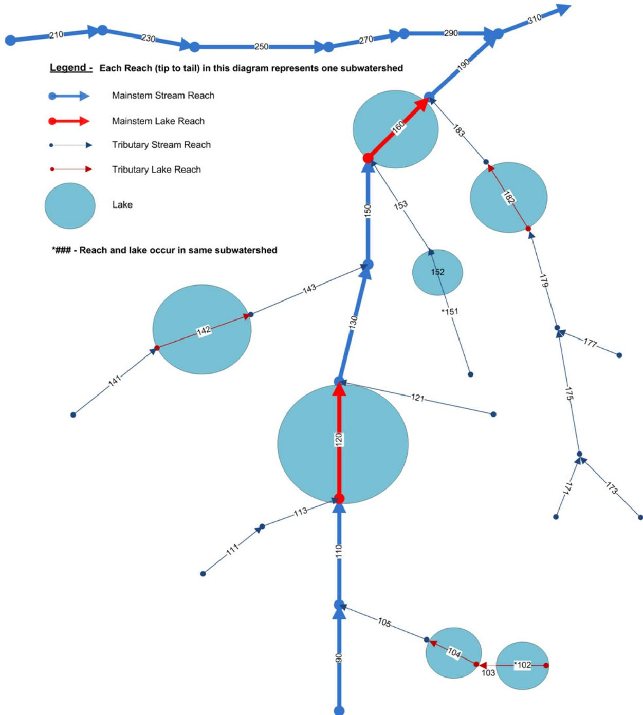
Figure 3. Reach Numbering Schematic.
