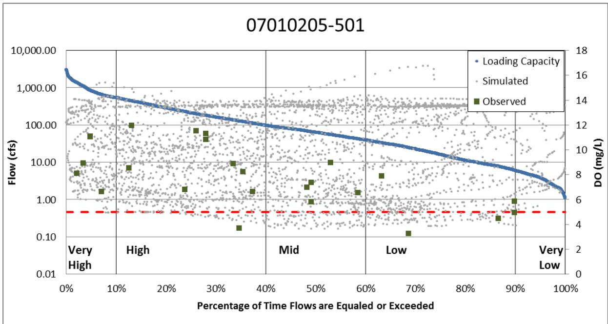
Figure 3-11. Dissolved oxygen samples taken before 9:00 a.m. in Buffalo Creek plotted on flow duration curve. The red dashed line indicates the 5 mg/L DO standard. Simulated DO values represent the daily minimum dissolved oxygen values.
