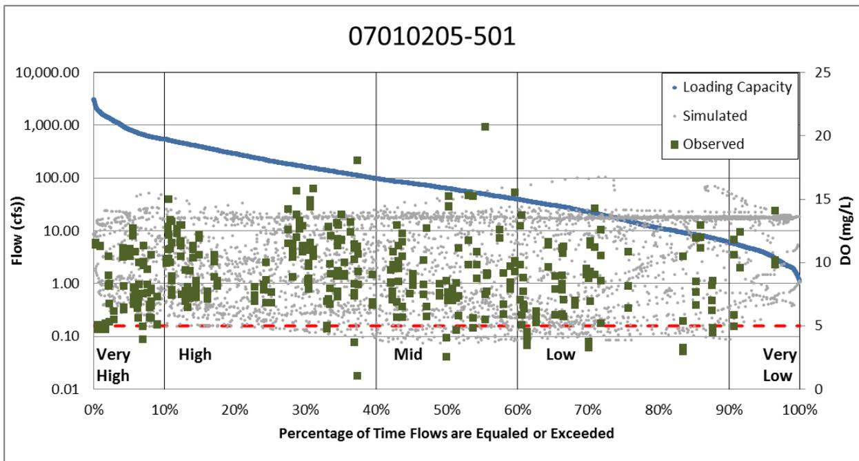
Figure 3-10. All dissolved oxygen samples in Buffalo Creek plotted on flow duration curve. The red dashed line indicates the 5 mg/L DO standard. Simulated DO values represent the daily minimum dissolved oxygen values.
