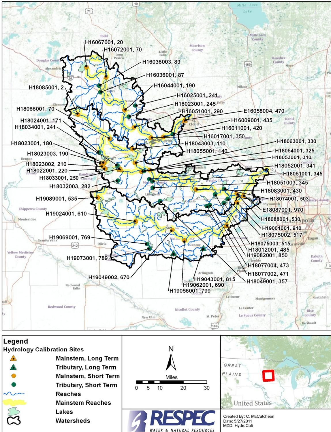
Figure 1. Flow Calibration Gages Within the Sauk and Crow Watersheds.
