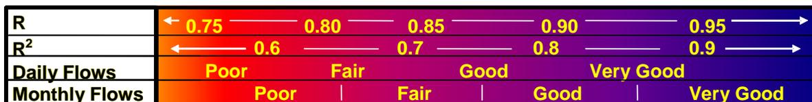
**Figure 14.** General Calibration/Validation  $R$  and  $R^2$  Targets for HSPF Applications.
