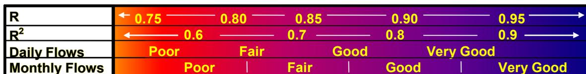
**Figure 8.** General Calibration/Validation *R* and *R*<sup>2</sup> Targets for HSPF Applications.
