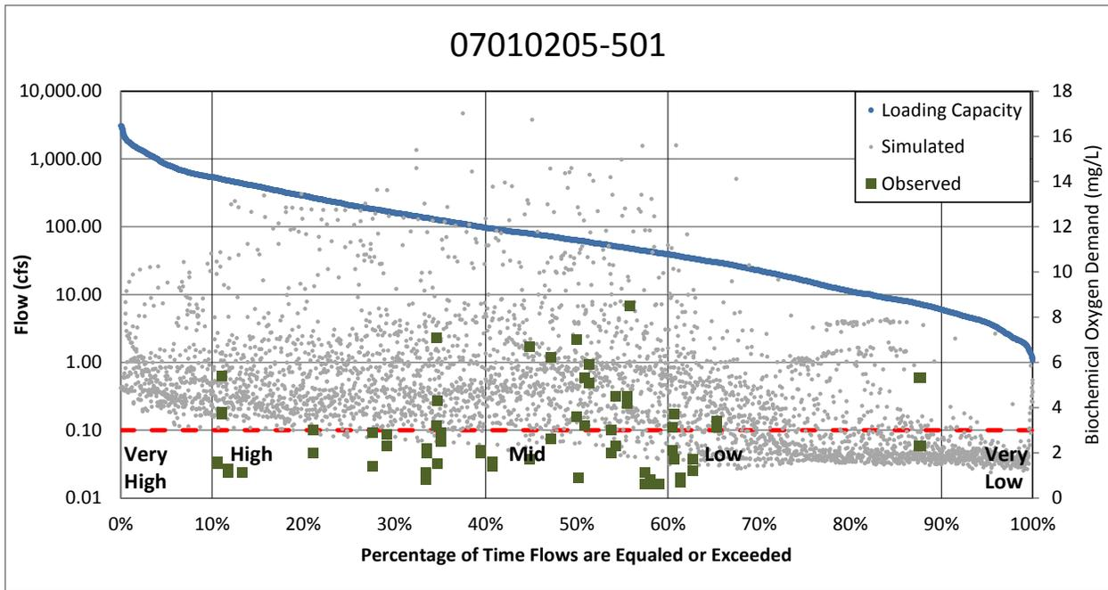
Figure 3-12. BOD5 samples in Buffalo Creek plotted on flow duration curve. The red dashed line indicates the 3 mg/L proposed BOD5 standard. Simulated BOD5 represent the daily average values.
