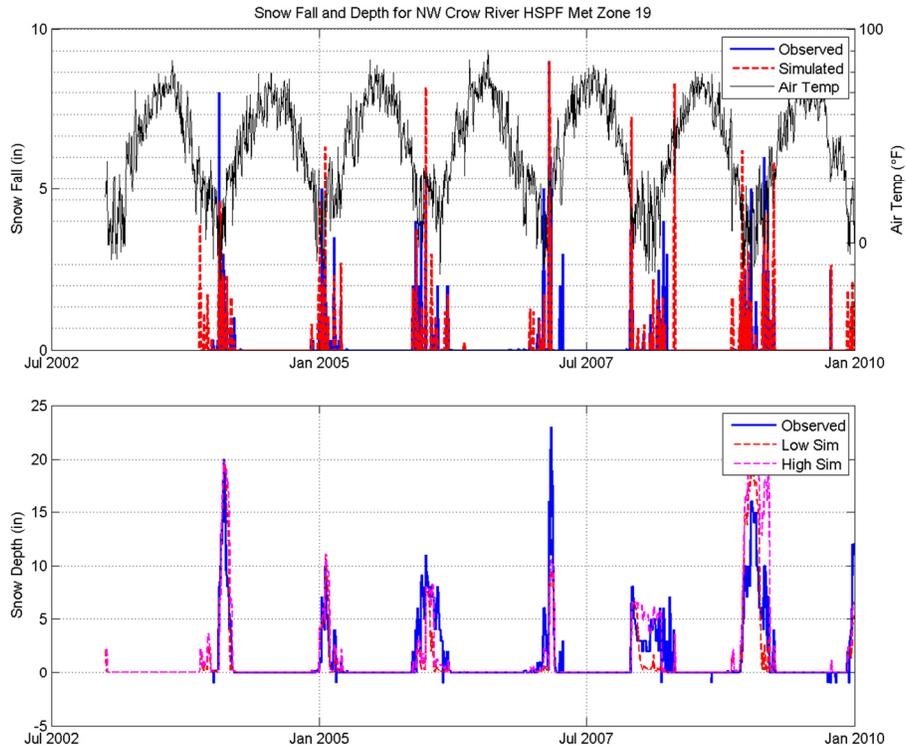
**Figure 3.** Snow Level (Top) and Snow Depth (Bottom) Calibration Figures.
