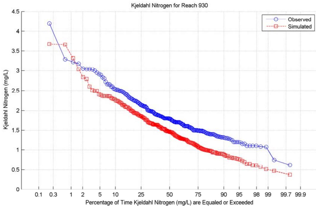
**Figure B-28.** Kjeldahl Nitrogen Concentration Duration Curve at Reach 930.
