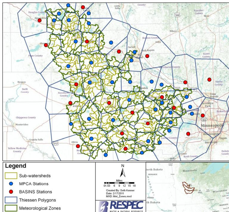
**Figure 2.** Aggregation of Subwatersheds Into Meteorological Zones Using the Thiessen Polygon Approach.
