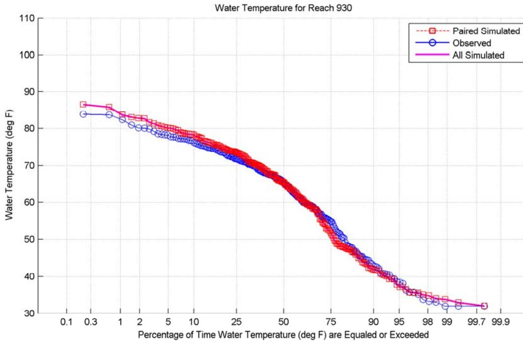
**Figure B-4.** Water Temperature Concentration Duration Curve at Reach 930.
