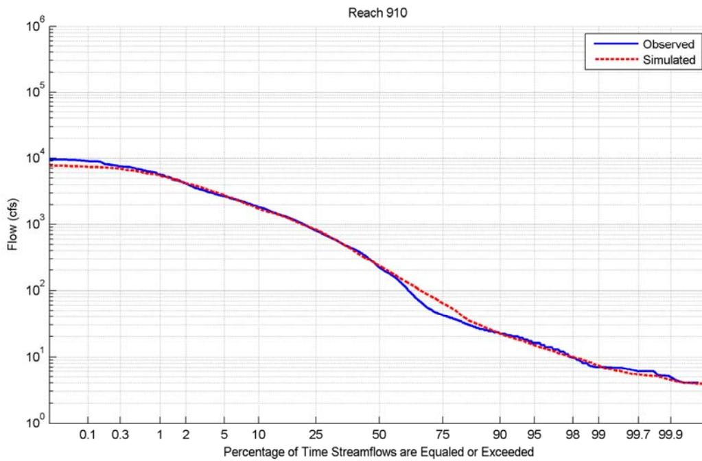
**Figure 13.** Flow-Duration Curve Example.
