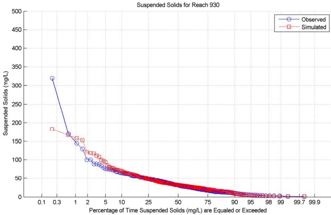
**Figure B-1.** Suspended Solids Concentration Duration Curve at Reach 930.
