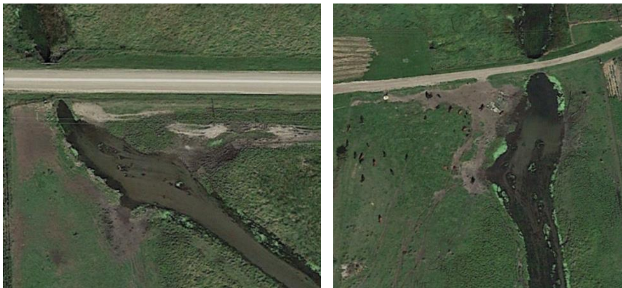
Figure 57. Channel over widening in Adley Creek due to cattle trampling.
