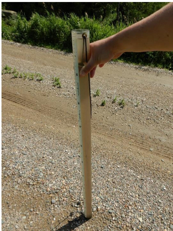
Figure 90. Secchi tube reading from Stony Creek after a storm event in July 2020.
