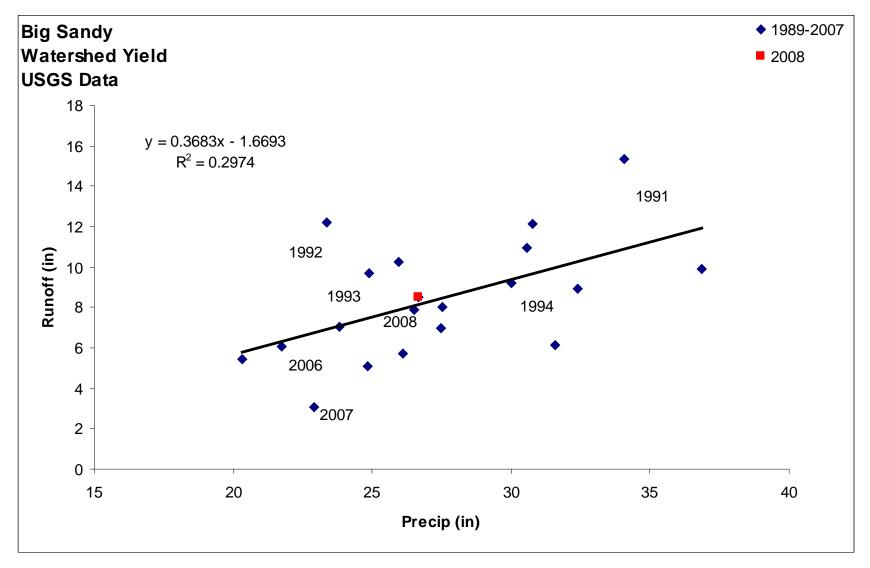
Figure 3-15 Relationship between precipitation and watershed yield calculated by the USGS using Big Sandy dam flows
