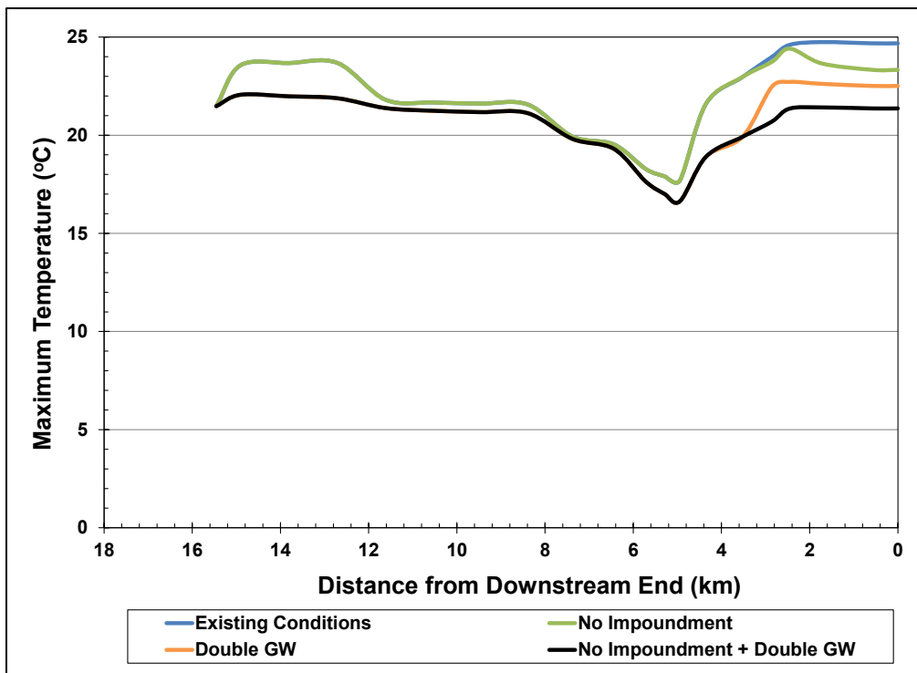
Figure B-20 Maximum Creek Temperatures for each QUAL2K model run on date 8/20/2008
