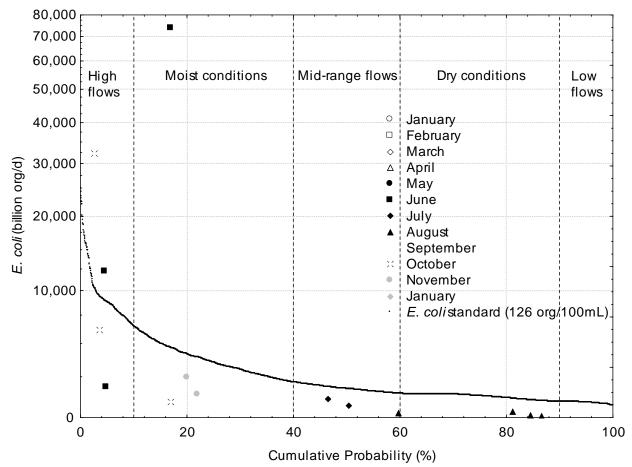
Figure 88. Load duration curve for *E. coli* at Rum River.
