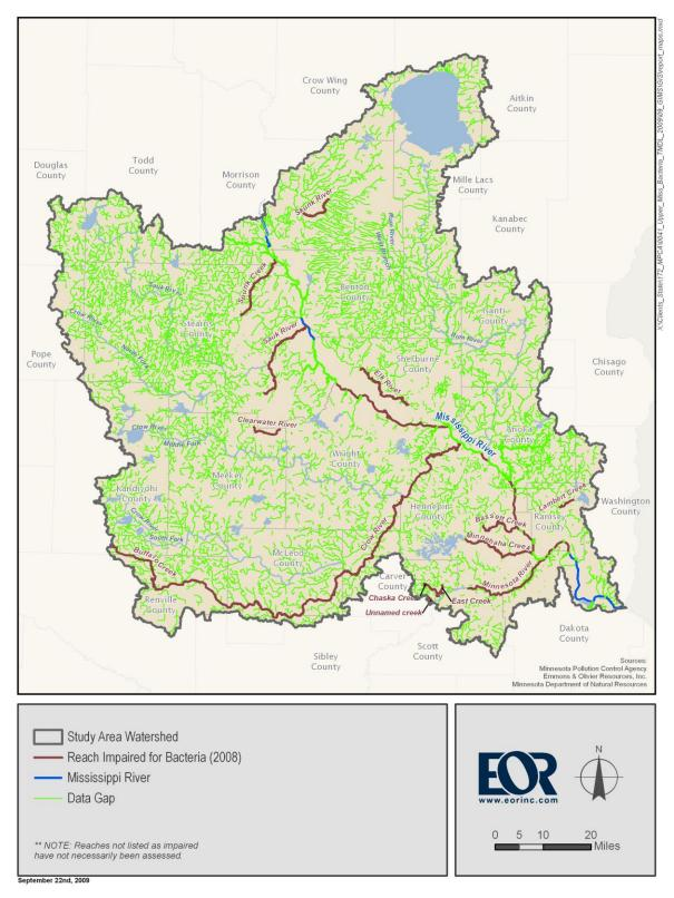
Figure 112. Mississippi River mainstem and tributary data gaps within the whole study area; those missing both *E. coli* and fecal coliform data.
