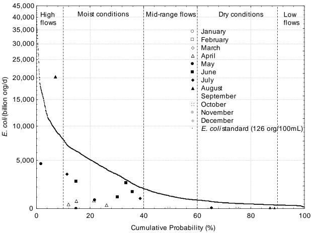
Figure 87. Load duration curve for *E. coli* at Crow River.
