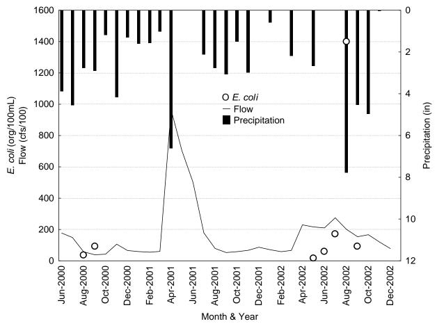
**Figure 60.** *E. coli* geometric means, mean flow and total precipitation at RM 839.7 from 2000-2002. Precipitation data unavailable from the following months: 2001 - May, June & December; 2002 - February, April, June, July & December.
