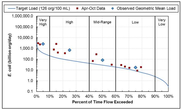
Figure A-11. E. coli load duration curve, Spring Branch Creek (AUID 07020010-574).
