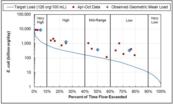
Figure A-12. E. coli load duration curve, Perch Creek (AUID 07020010-523).
