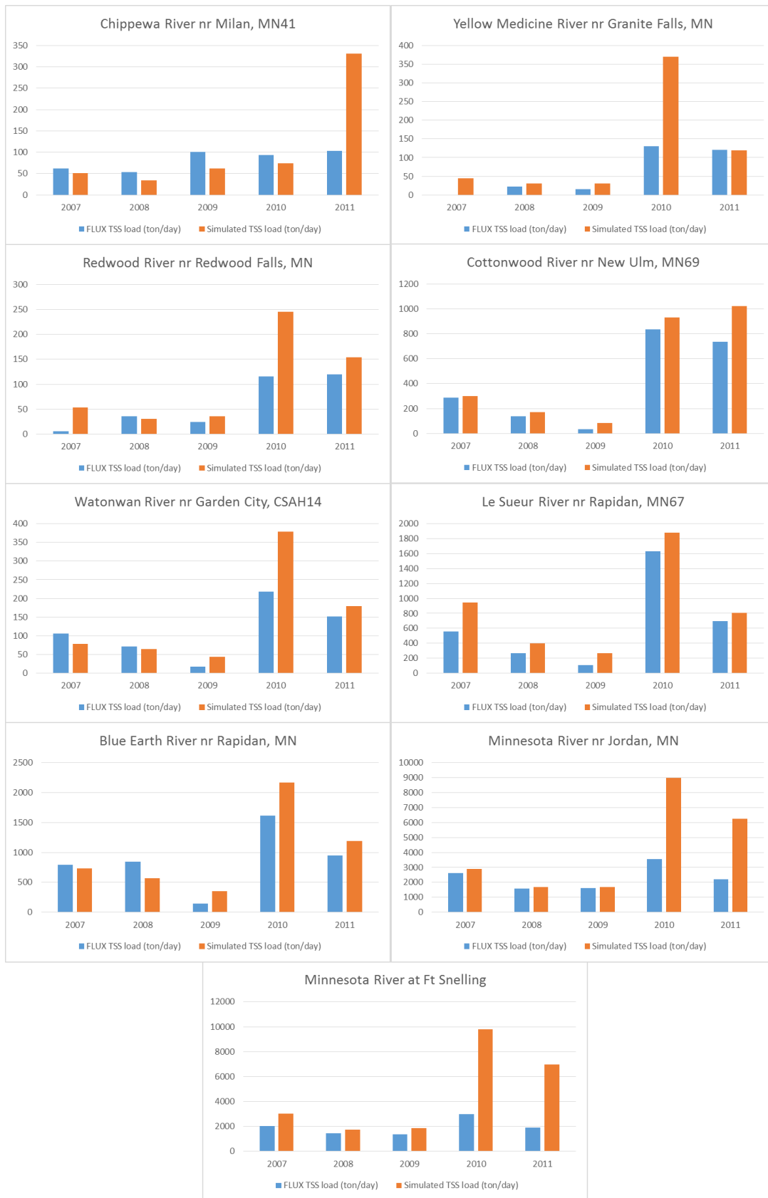
Figure 12. Comparison of Model and FLUX TSS Load Estimates, Calendar Years 2007 - 2011
