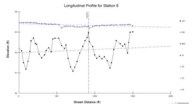
Figure 32. Longitudinal Profile for Station 8 on the Cedar River.
