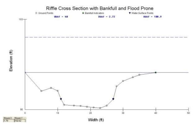
Figure 36. Riffle Cross Section for Station 11 on the Cedar River
