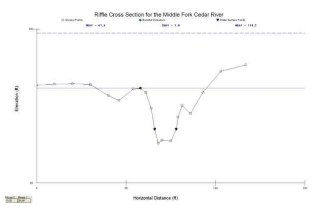
Figure 81. Riffle Cross Section with bankfull and flood prone for the Middle Fork Cedar River
