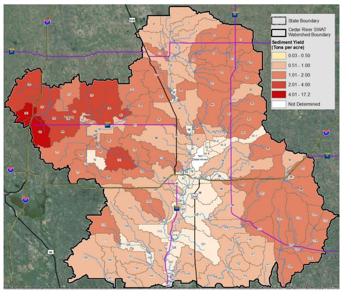
**Figure 9.** SWAT model upland sediment yield estimates without BMPs implemented in the Cedar River watershed.
