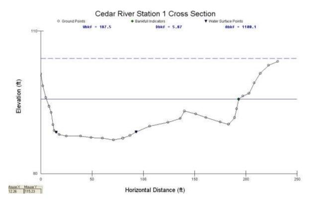
Figure 1. Riffle Cross Section at Station 1 upstream of CR 105.
