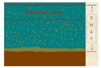
Figure 4. Depiction of water quality monitoring zone relative to sediment modeling in SWAT.
