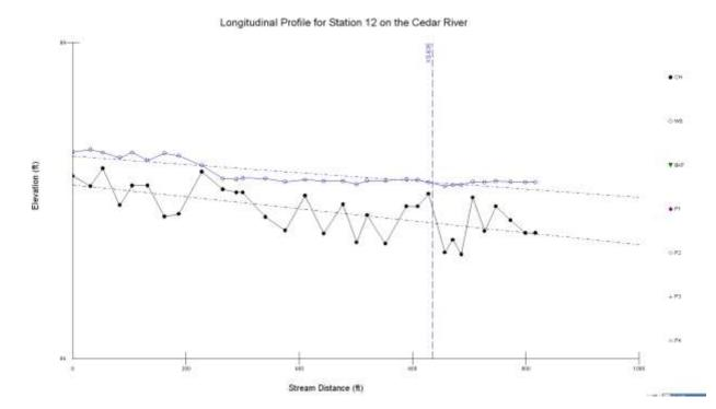
Figure 42. Longitudinal Profile for Station 12 on the Cedar River
