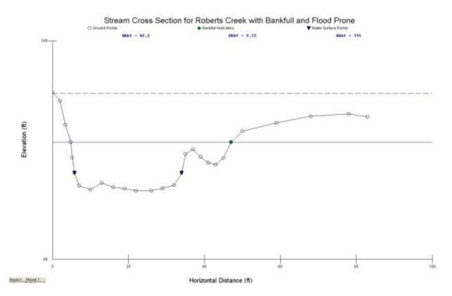
Figure 76. Riffle Cross Section with Bankfull and Flood Prone for Roberts Creek.
