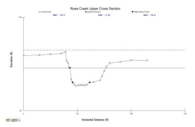
Figure 51. Riffle Cross Section with Bankfull and Flood Prone Area for Upper Rose Creek
