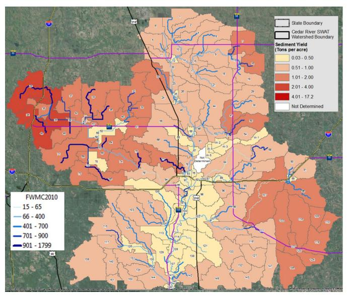
**Figure 10.** SWAT model upland sediment yield and flow-weighted mean sediment concentration estimates for reaches in the Cedar River watershed.
