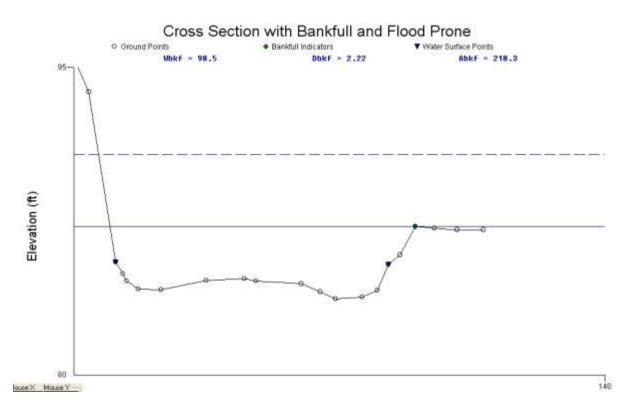
Figure 31. Riffle Cross Section for Station 8 on the Cedar River.
