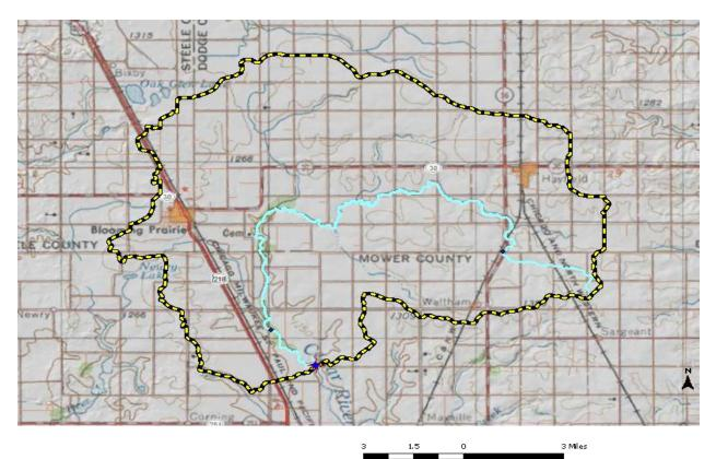
Figure 34.. Watershed (113 square miles) used in the USGS StreamStat Regession Flow Calaulations for Station 8.
