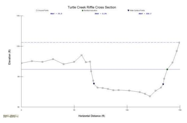
Figure 61. Riffle Cross Section with Bankfull and Flood Prone area for Turtle Creek
