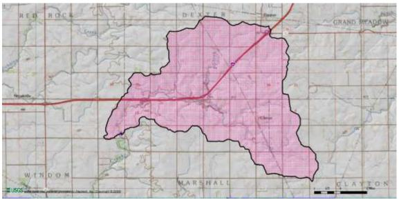
Figure 54.. Watershed (26.4 square miles) used in the USGS StreamStat Regession Flow Calaulations for Upper Rose Creek.
