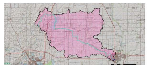
Figure 64. Watershed (152 square miles) used in the USGS StreamStat Regession Flow Calaulations for Turtle Creek.
