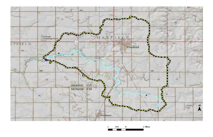
Figure 39.. Watershed (25 square miles) used in the USGS StreamStat Regession Flow Calaulations for Station 11
