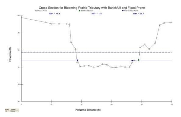
Figure 71. Riffle cross section for Blooming Prairie Creek with Bankfull and Flood Prone.
