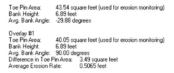
Figure 30. Erosion Loss and Erosion Rate for Study Bank at Site 7 on the Cedar River
