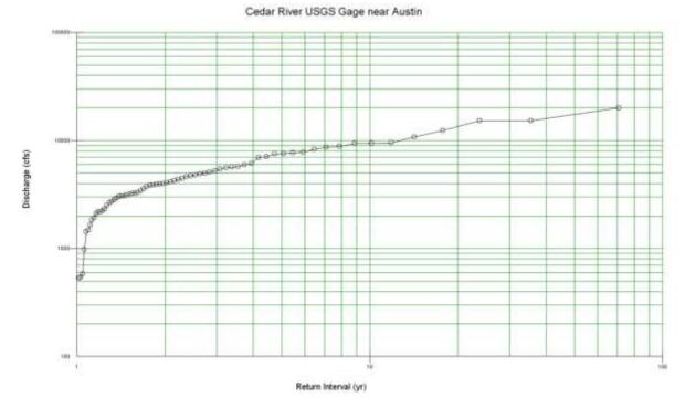
Figure 16.USGS Gage Analysis for the Cedar River below Austin which has a 1.5 year event of 2922 CFS.
