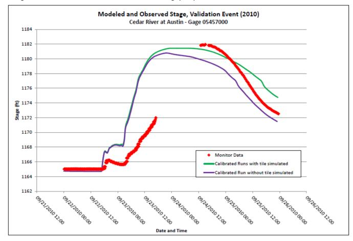
Figure 14 – Cedar River at Austin Modeled and Observed Stage (2010)
