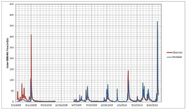
*Figure 2: Observed streamflow volume (red) and SWAT simulated streamflow (blue) on the Cedar near Austin between 2008 and 2010. (Figure produced by Barr.)*
