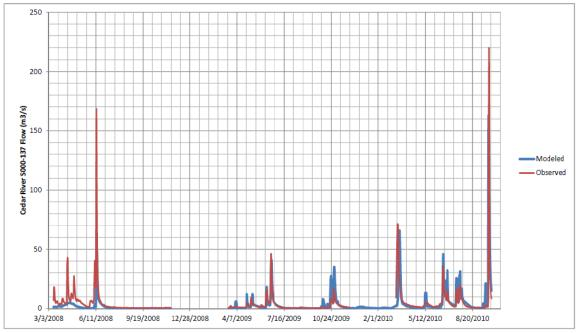
Figure 3. SWAT model flow calibration results for the Upper Cedar River station.
