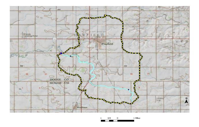
Figure 44.. Watershed (20 square miles) used in the USGS StreamStat Regession Flow Calaulations for Station 12
