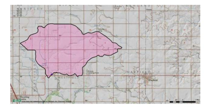
Figure 84. Watershed (18.7 square miles) used in the USGS StreamStat Regession Flow Calaulations for the Middle Fork Cedar River
