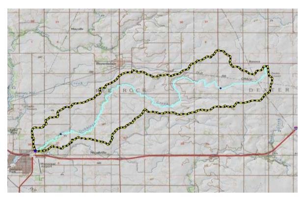
Figure 49.. Watershed (19 square miles) used in the USGS StreamStat Regession Flow Calaulations for Dobbins Creek near Austin.
