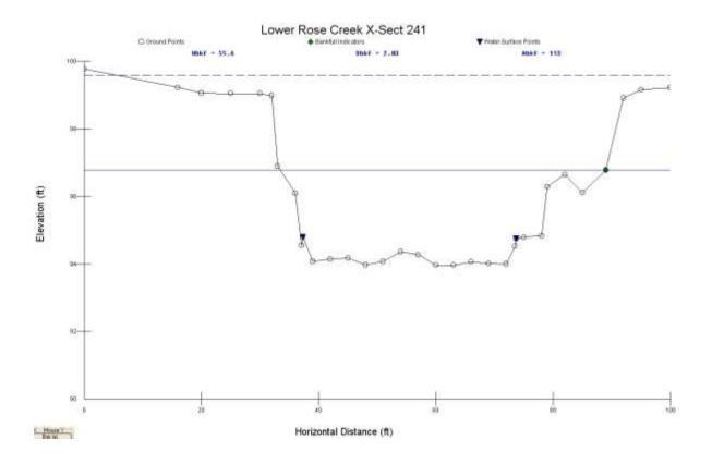
Figure 56. Riffle Cross Section for Lower Rose Creek with Bankfull and Flood Prone.
