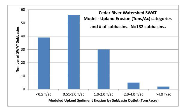
Figure 1. Frequency distribution of the subbasins in the Cedar River Watershed with modeled SWAT upland sediment erosion data for calendar year 2010.
