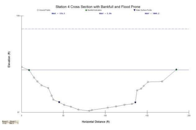
Figure 18. . Riffle Cross Section at Station 4 on the Cedar River.
