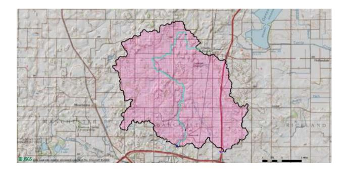
Figure 69. Watershed (26 square miles) used in the USGS StreamStat Regession Flow Calaulations for Bancroft Creek.
