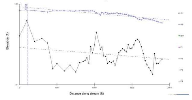
Figure 2. Longitudinal Stream Profile for 1800 feet of Station 1.
