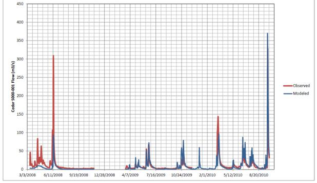
Figure 1. SWAT model flow calibration results for the Cedar River station near Austin, MN.
