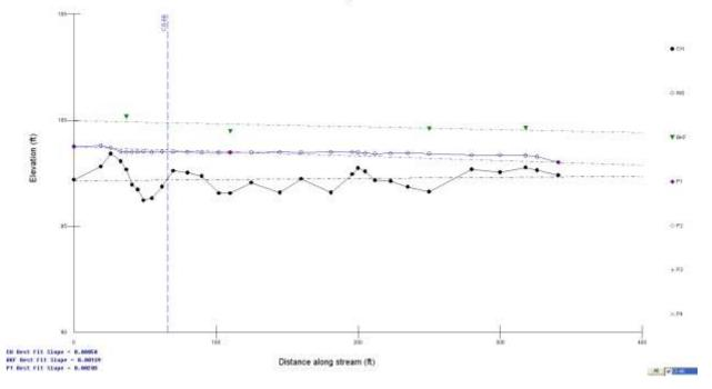
Figure 47. Longitudinal Profile for Dobbins Creek near Austin
