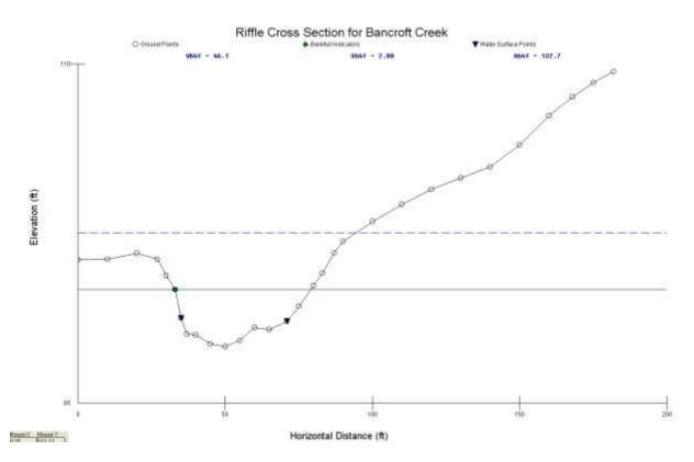
Figure 66. Riffle Cross Section with Bankfull and Flood Prone for Bancroft Creek
