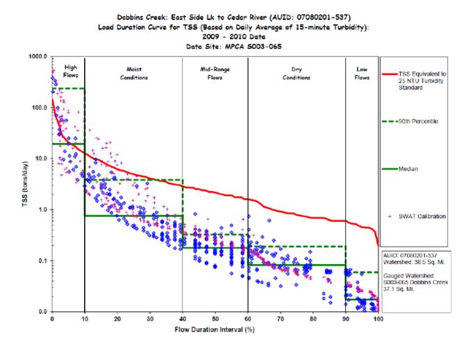
Figure 7. Dobbins Creek TSS load duration curve and calibrated SWAT model sediment loads.
