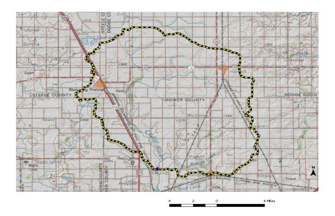
Figure 26. Watershed (160 square miles) used in the USGS StreamStat Regession Flow Calaulations for Sation 7.
