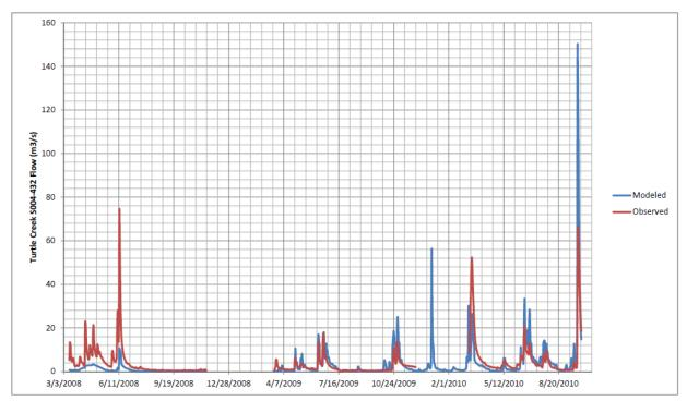
Figure 2. SWAT model flow calibration results for the Turtle Creek station near Austin, MN.
