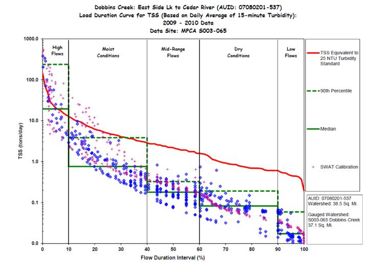
Figure 7. Dobbins Creek TSS load duration curve and calibrated SWAT model sediment loads.
