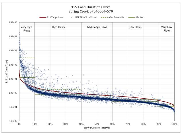
Figure 41. ZUMBRO RIVER HUC-10: Load Duration Curve with HSPF model predicted TSS loads for Spring Creek – 07040004-570. WQ Standard is 10 mg/L
