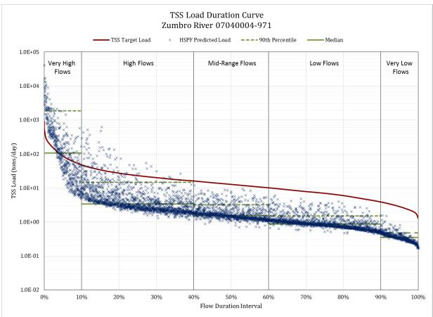
Figure 37. NORTH FORK ZUMBRO RIVER HUC-10: Load Duration Curve for Zumbro River – 07040004-971. WQ Standard is 65 mg/L.
