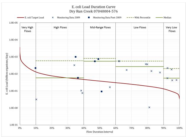
Figure 33. ZUMBRO RIVER HUC-10: Load Duration Curve for Dry Run Creek – 07040004-576.
