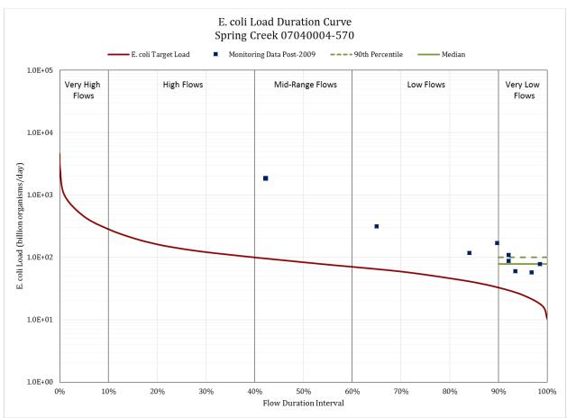
Figure 30. ZUMBRO RIVER HUC-10: Load Duration Curve for Spring Creek – 07040004-570.
