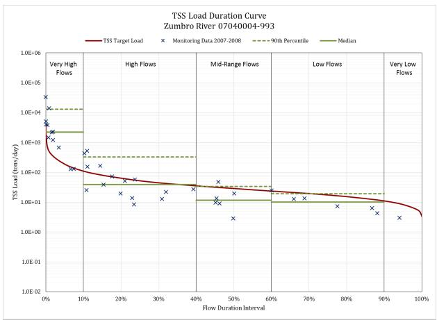
Figure 36. MIDDLE FORK ZUMBRO RIVER HUC-10: Load Duration Curve for Zumbro River – 07040004-993. WQ Standard is 65 mg/L.
