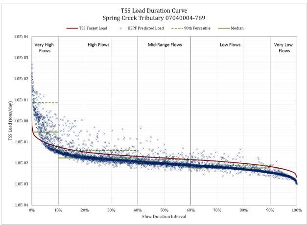
Figure 43. ZUMBRO RIVER HUC-10: Load Duration Curve for Spring Creek Tributary – 07040004-769. WQ Standard is 10 mg/L.
