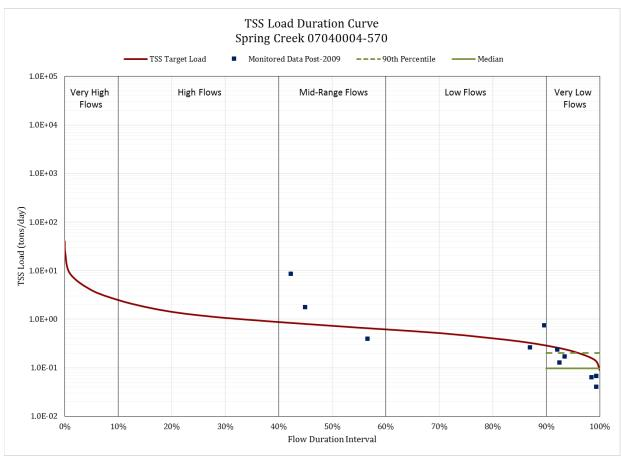
Figure 42. ZUMBRO RIVER HUC-10: Load Duration Curve with water quality data TSS loads for Spring Creek – 07040004-570. WQ Standard is 10 mg/L.
