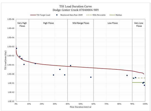
Figure 39. SOUTH BRANCH MIDDLE FORK ZUMBRO RIVER HUC-10: Load Duration Curve with water quality data TSS loads for Dodge Center Creek – 07040004-989. WQ Standard is 65 mg/L.
