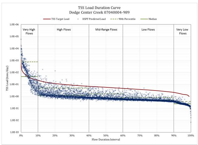
Figure 38. SOUTH BRANCH MIDDLE FORK ZUMBRO RIVER HUC-10: Load Duration Curve with HSPF model predicted TSS loads for Dodge Center Creek – 07040004-989. WQ Standard is 65 mg/L.
