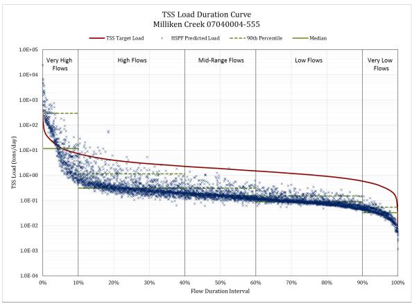
Figure 35. MIDDLE FORK ZUMBRO RIVER HUC-10: Load Duration Curve for Milliken Creek – 07040004-555. WQ Standard is 65 mg/L.
