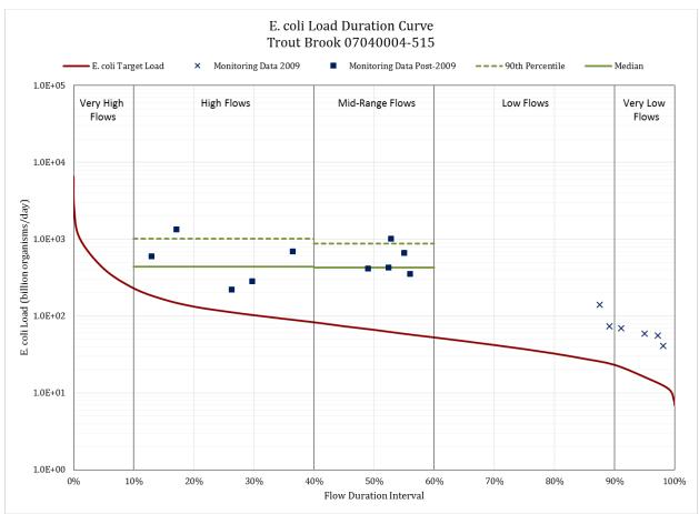
Figure 20. NORTH FORK ZUMBRO RIVER HUC-10: Load Duration Curve for Trout Brook – 07040004-515.
