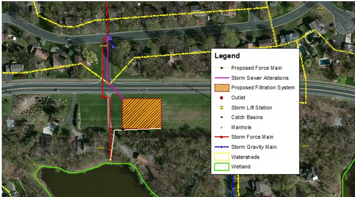
Figure 5.24. Stormwater reroute with underground and basin iron enhanced filtration system project alternatives for Watershed LP-53.
