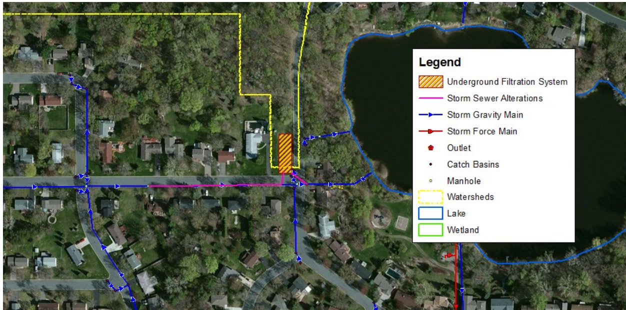
Figure 5.23. Stormwater reroute with an underground filtration system.
