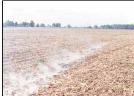
In Ohio, Shipitalo and Gibbs pump smoke into a tile line to show the connectivity of the surface to tile line.
