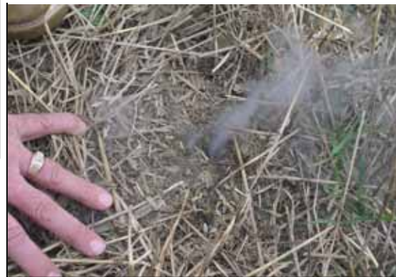
Figure 8.2.2 – Examples of macropore/preferential flow routes in a no till tiled field in Ohio
