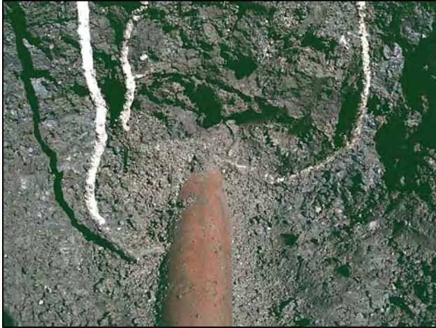
The pictures depict a conventionally tilled, clayey soil where earthworms appear to preferentially burrow towards the drains. The tile in this photo is 4 feet deep.
