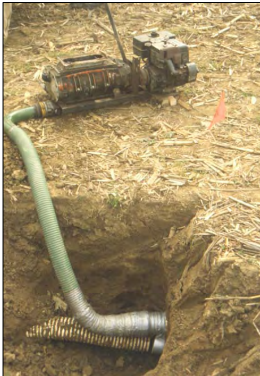
In Ohio, Shipitalo and Gibbs pump smoke into a tile line to show the connectivity of the surface to tile line.
