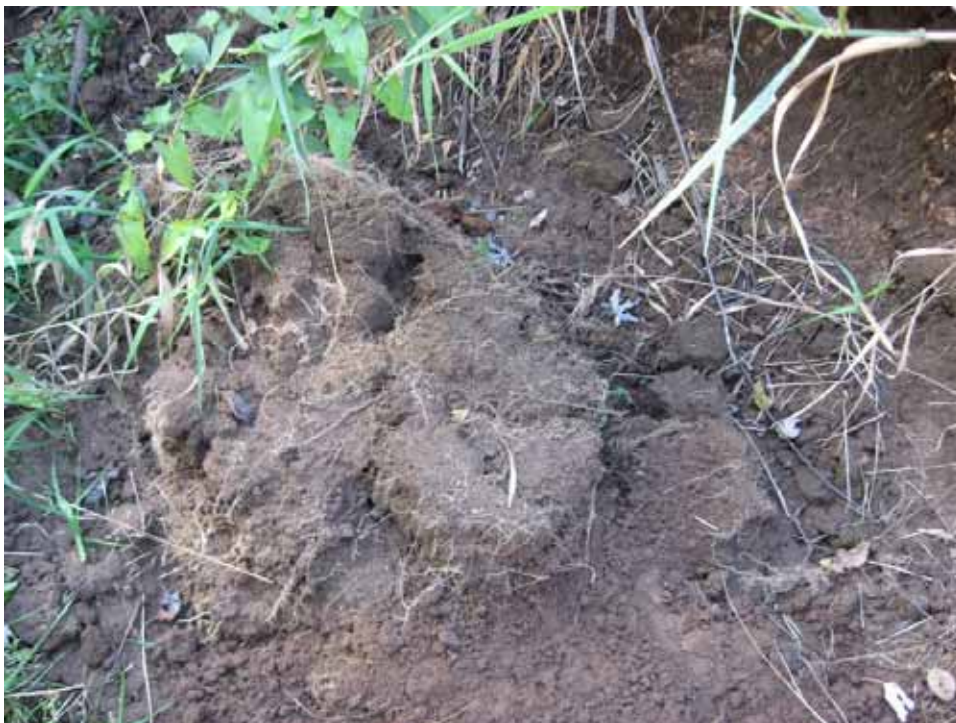
Close-up view of the streambank material where the failure block is separating as shown in the previous two photos.
