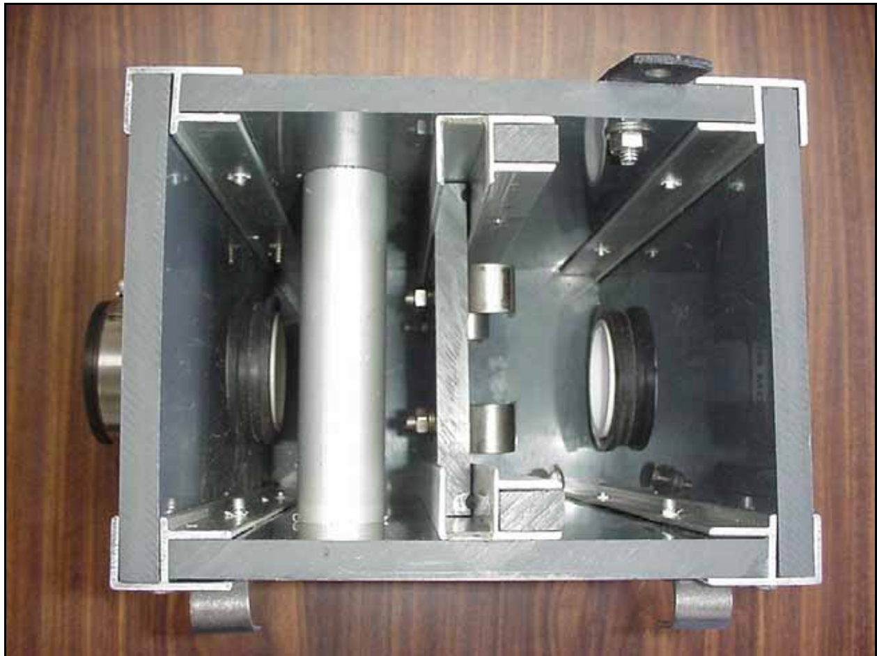
Figure 7. Interior View of a Drainage Control Structure with Adjustable Baffle Height
