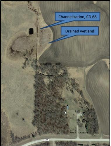
Figure 4-72. Portion of CD 68 (AUID 655), between CSAH 29 and CSAH 3, which was dug through the middle of a wetland
