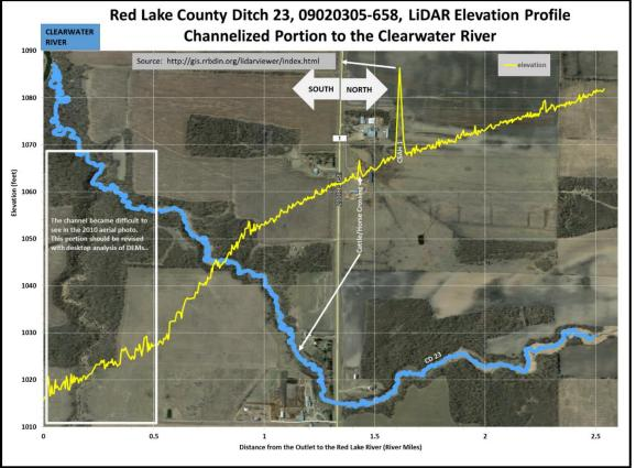
Figure 4-51. Longitudinal LiDAR profile of the CD 23 channel (AUID 658)
