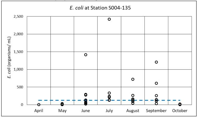
Figure 3-7: *E. coli* sampling aggregated by month on Hay Creek at the monitoring station S004-135. The dashed line denotes the stream water quality standard (126 org/100mL).
