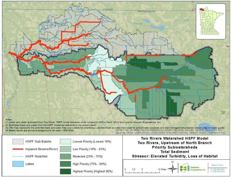
Figure 3-19: Subwatershed priority of TSS yields for Two Rivers, Middle Branch Two Rivers to North Branch Two Rivers (AUID 09020312-501) drainage area based on HSPF model result.
