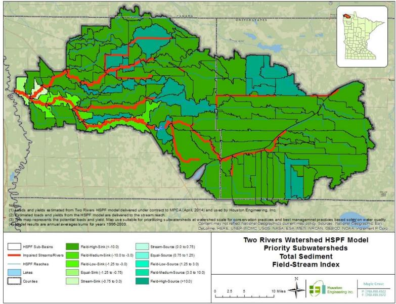
Figure 3-17: Total Sediment Field Stream Index using HSPF model results.
