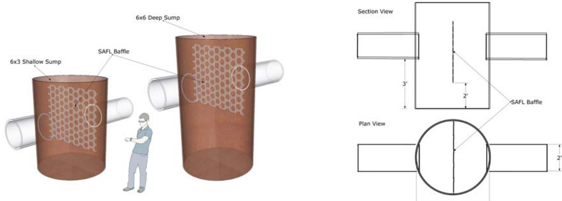
Figure 4.7. The SAFL Baffle is installed in a sump manhole to minimize resuspension of pollutants collected in the sump.
