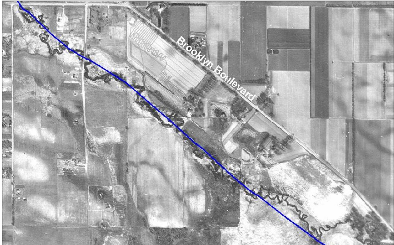
Figure 2.5. 1947 aerial photo of Shingle Creek at Zane Avenue in Brooklyn Park. Note: The blue line is the current stream alignment, constructed in 1960
