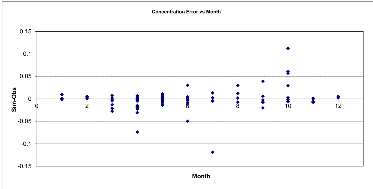
Figure 301. Residual (Simulated - Observed) vs. Month Total Phosphorus (TP) at Poplar River near Lutsen
