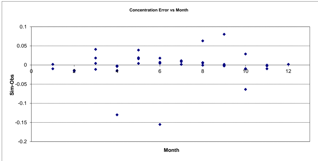
Figure 311. Residual (Simulated - Observed) vs. Month Ammonia Nitrogen (NH3) at Brule River near Hovland
