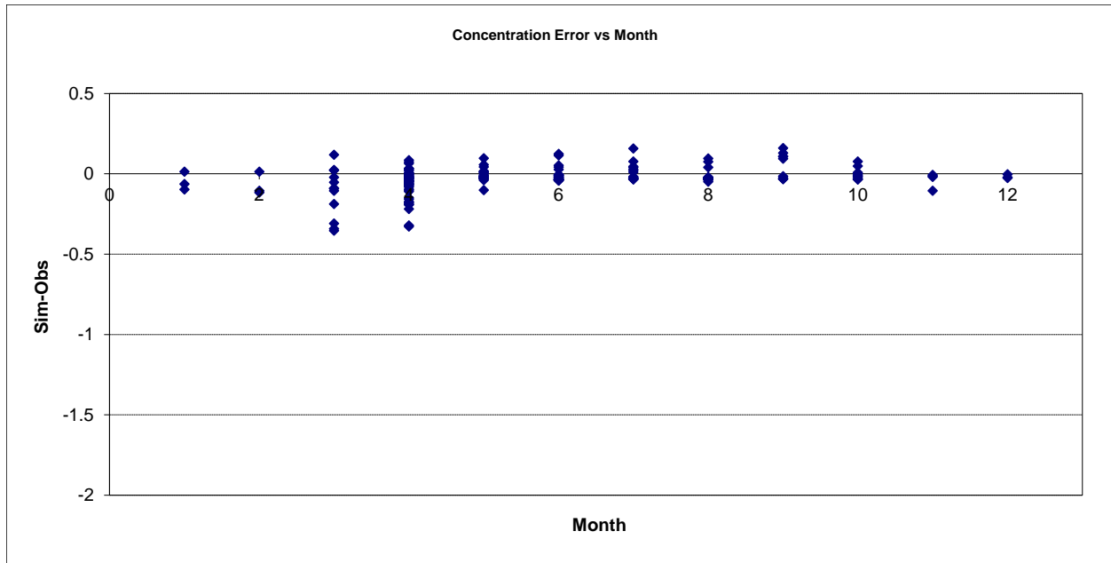
Figure 114. Residual (Simulated - Observed) vs. Month Nitrite+ Nitrate Nitrogen (NOx) at Sucker River near Palmers
