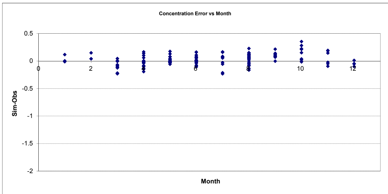
Figure A-141. Residual (Simulated - Observed) vs. Month Nitrite+ Nitrate Nitrogen (NOx) at St. Louis River at Scanlon, MN (03174001)
