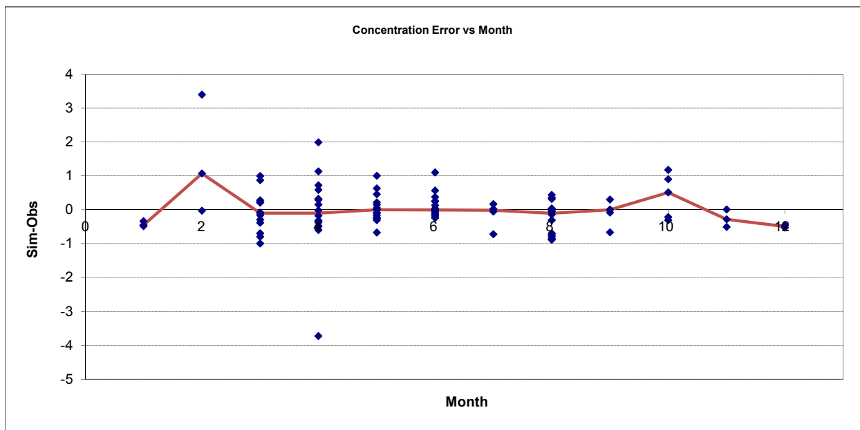
Figure B-188. Residual (Simulated - Observed) vs. Month Total Nitrogen (TN) at Nemadji River nr South Superior, WI (05011002)
