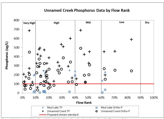
Figure 3-5. Unnamed Creek and Mud Lake TP and orthophosphate data by flow condition.
