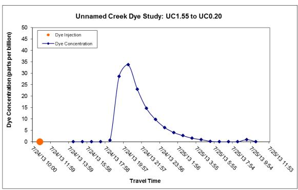
Figure 1-3. UC1.55 to UC0.20 dye study measurements.
