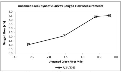
Figure 1-4. Gauged flow measurements during the July 24 synoptic survey.
