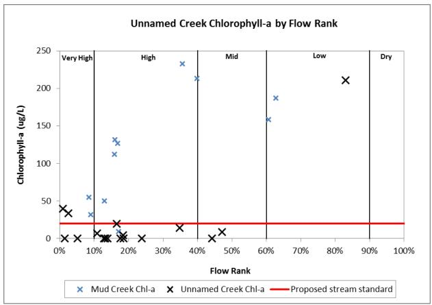
Figure 3-7. Unnamed Creek and Mud Lake chlorophyll- $\alpha$  data by flow condition. Note: Samples below detection limit (<5  $\mu$ g/L) are shown on the figure as 0  $\mu$ g/L.
