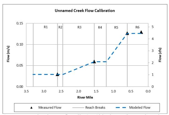
Figure 1.2. Unnamed Creek QUAL2K flow calibration with headwater, tributary and groundwater diffuse inflows.
