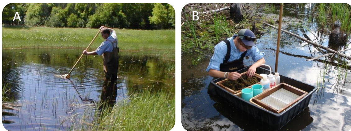
Figure 5. Aquatic macroinvertebrate sample collection was a two-step process involving (A) dip nets to collect organisms and vegetative material from the emergent zone, and (B) hardware cloth with pans underneath to separate collected macroinvertebrates from the detritus.
