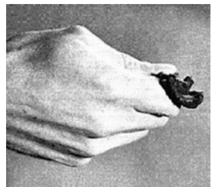
Fig. 5 Medium-textured soil does not form ribbons. Medium textured soil feels fairly smooth and floury. Dry clods are readily
