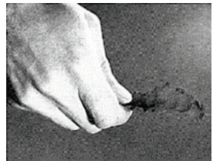
Fig. 4: Fine-textured soil forms a long, shiny pliable ribbon. The moist ribbon feels smooth and sticky. Dry clods are very hard.
